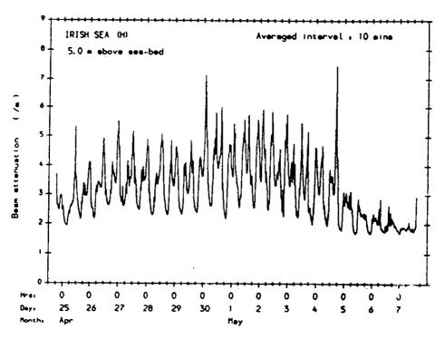
Figure 3. Beam attenuation recorded by moored transmissometers at 1, 5 and 15m above the sea bed at the central observation site (site G, upper plot) and at 5m above the sea bed at the southerly observation site (site H, lower plot).
