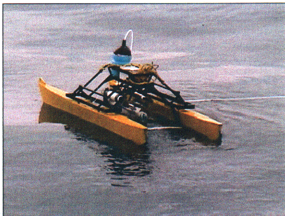
Plate 3. Glass Rotating Drum sampling of sea surface microlayer.
