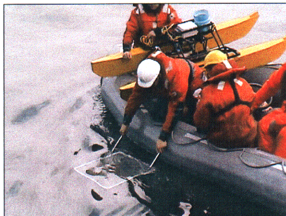
Plate 4. Garrat Screen sampling of sea surface microlayer.
