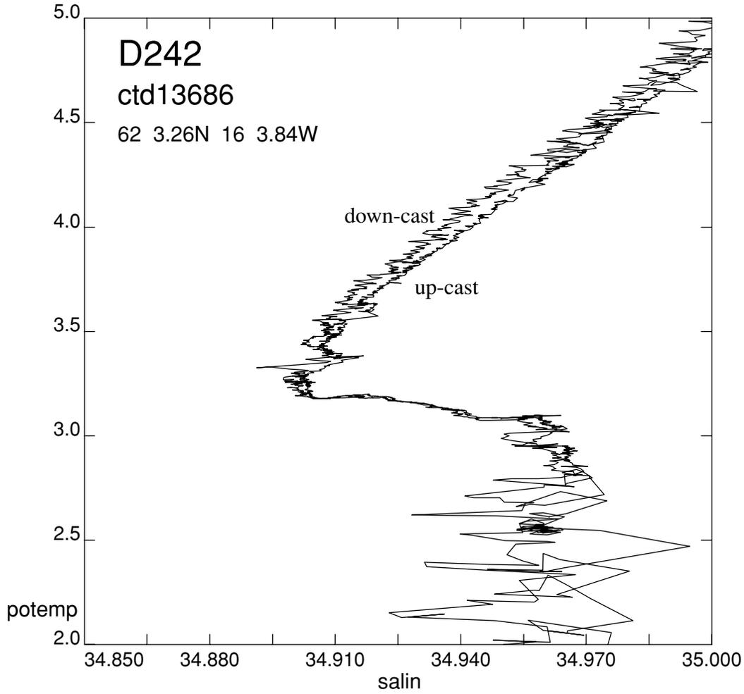
Figure 7 - D242 Station 13686, the first deep station with the replacement conductivity cell in DEEP04.
