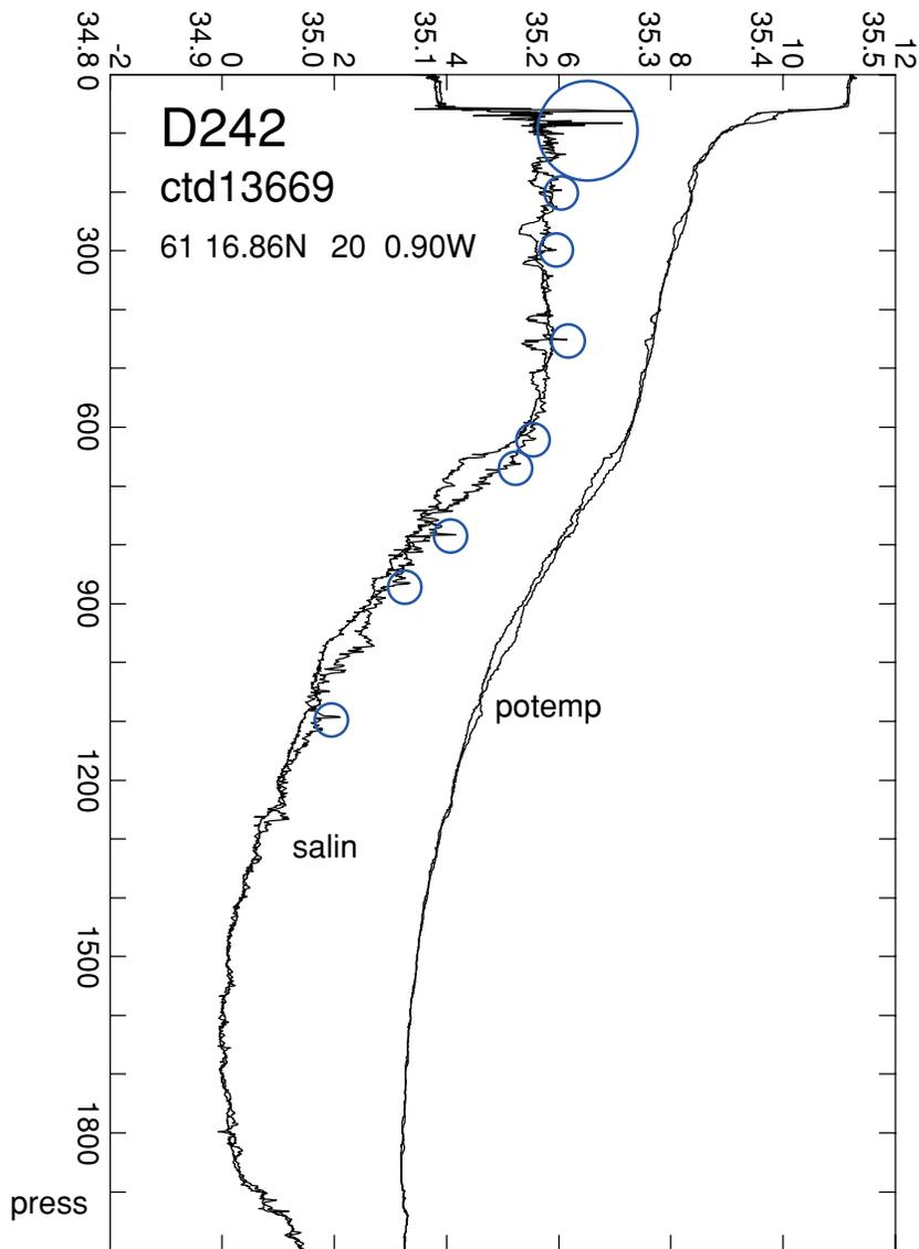
Figure 1 -Temperature and Salinity profiles from 3 cruises in approximately the same location. Data shown are 1hz data from up and down-casts; a) D242 Station 13669 with examples of spikes highlighted by circles.
