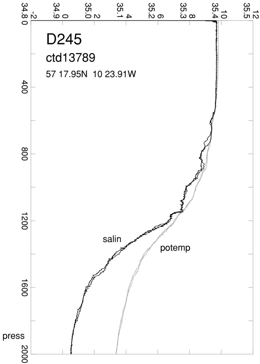
Figure 4 - Temperature and Salinity for D245 station 13789 showing the clean up and down profiles collected with the modified CTD frame and long LADCP.
