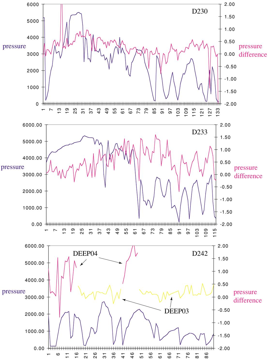
Figure 11 - Pressure differences between the on-deck readings before and after each cast on D230 (DEEP01, pressure corrected for hysteresis), D233 (DEEP04) and D242 (DEEP03 and DEEP04). Maximum pressure of each cast is also shown in blue.
