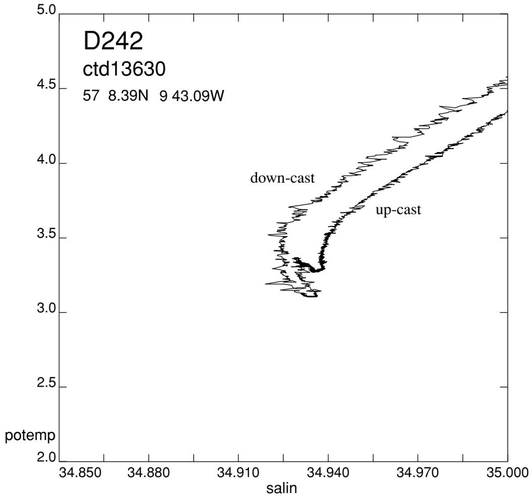
Figure 5 - D242 Station 13630, the test station, showing two jumps to higher salinity; at the bottom of the cast, and during an extended winch-stopped period.
