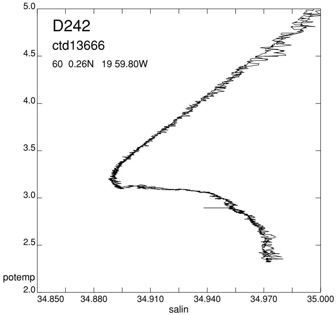
Figure 8 - D242 Station 13666, using DEEP03 and showing no hysteresis.
