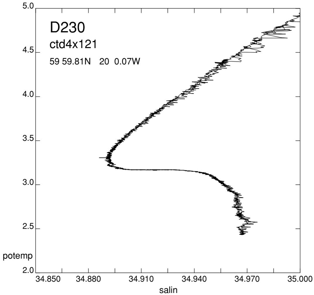
Figure 9 - D230 Station 121 using DEEP01 and showing no hysteresis.
