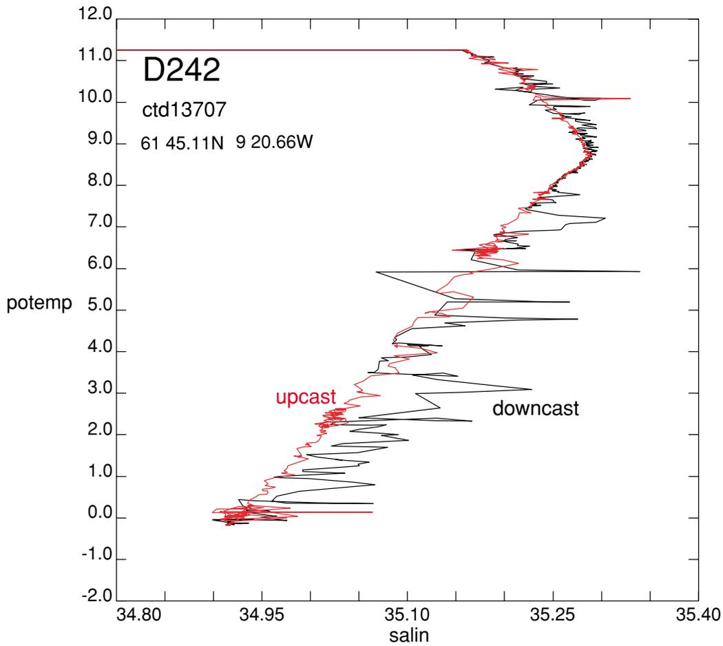
Figure 2a - Temperature-salinity plot for D242 station 13707 in the Faroe Bank Channel with very strong salinity and temperature gradient producing very bad spiking in the deep water. Data shown are 1hz; down-cast is in black, up-cast in red.
