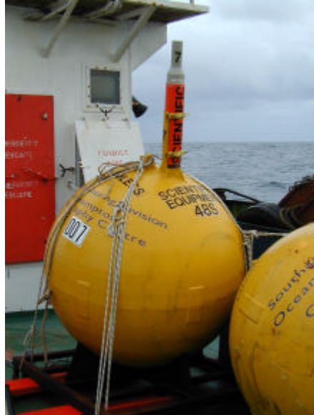
48 inch steel sphere fitted with OED ARGOS beacon
