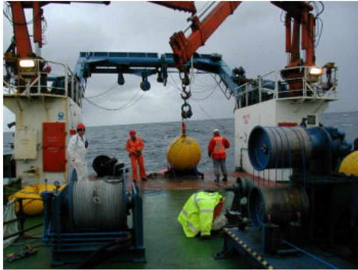
Machinery in readiness to deploy 48 inch steel sphere . Note use of both starboard and port cranes
