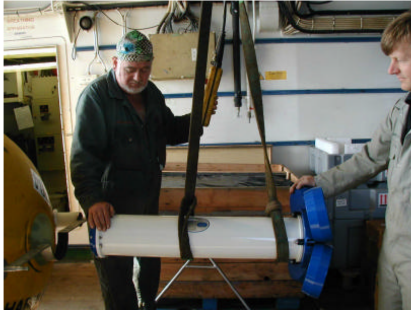
Rhys Roberts controlling the insertion of the LongRanger ADCP into the Syntactic buoy. Note removal of in line frame is required.
