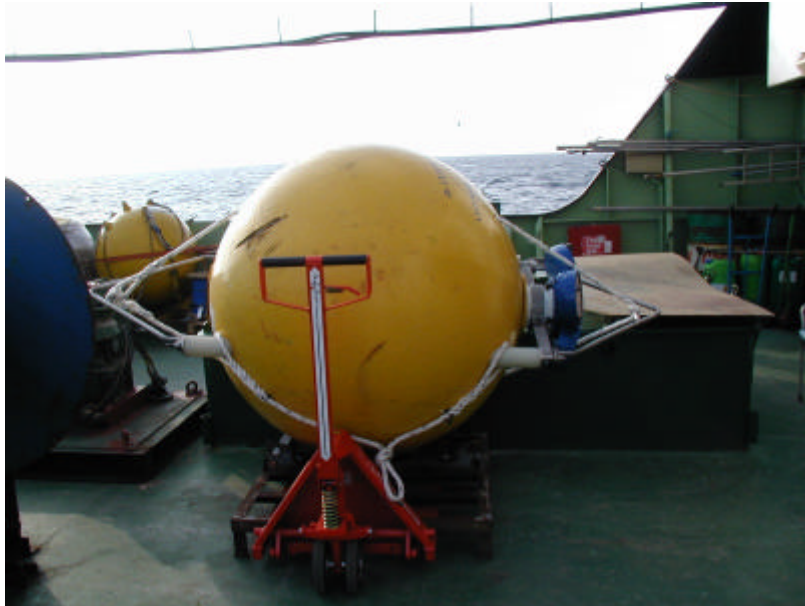
Syntactic Buoy fitted with Through Load framework. Instrument mounted is a Long Ranger ADCP.
