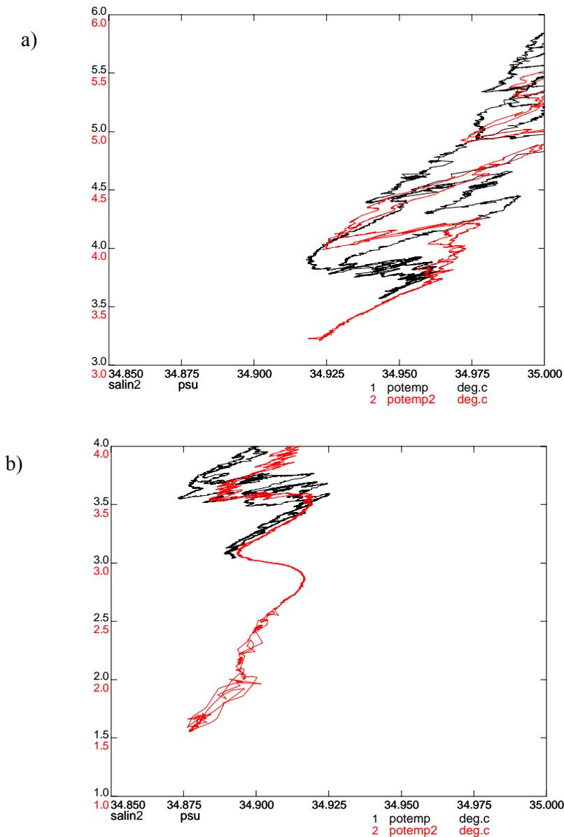
**Fig 14.** Small scale comparison of the T/S relation for the ARIES and lowered CTD SeaBird sensors for (a) stations 15091 (ARIES in black) and 15085 (lowered in red), and (b) stations 15106 (ARIES in black) and 15100 (lowered in red).
