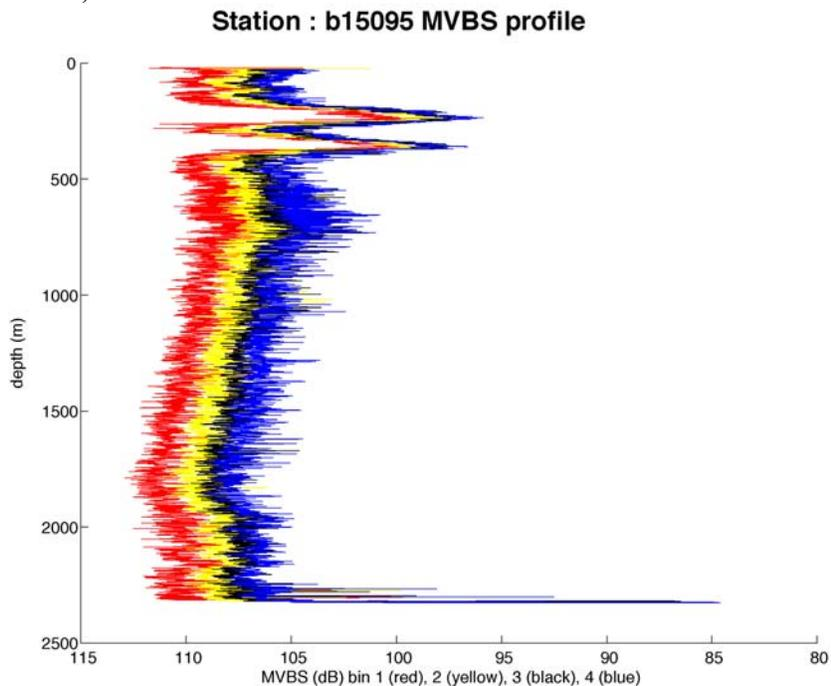
**Fig 17.** Typical 600 kHz acoustic backscatter data (station 15095).
