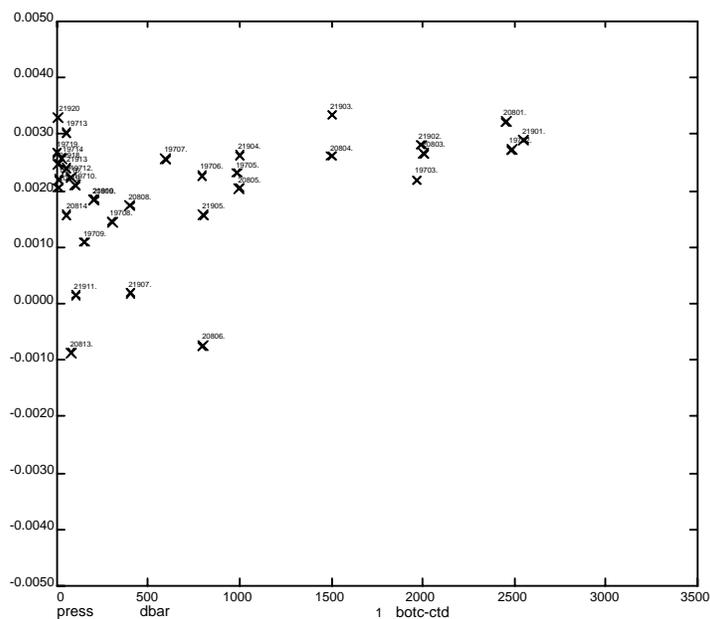
**Fig 13.** Residual conductivity for stations 15197, 15208 and 15219.
