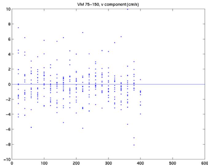
**Fig 19.** On station velocity profile difference between the two VM-ADCPs (75Khz-150Khz); a) East component, b) North component.
