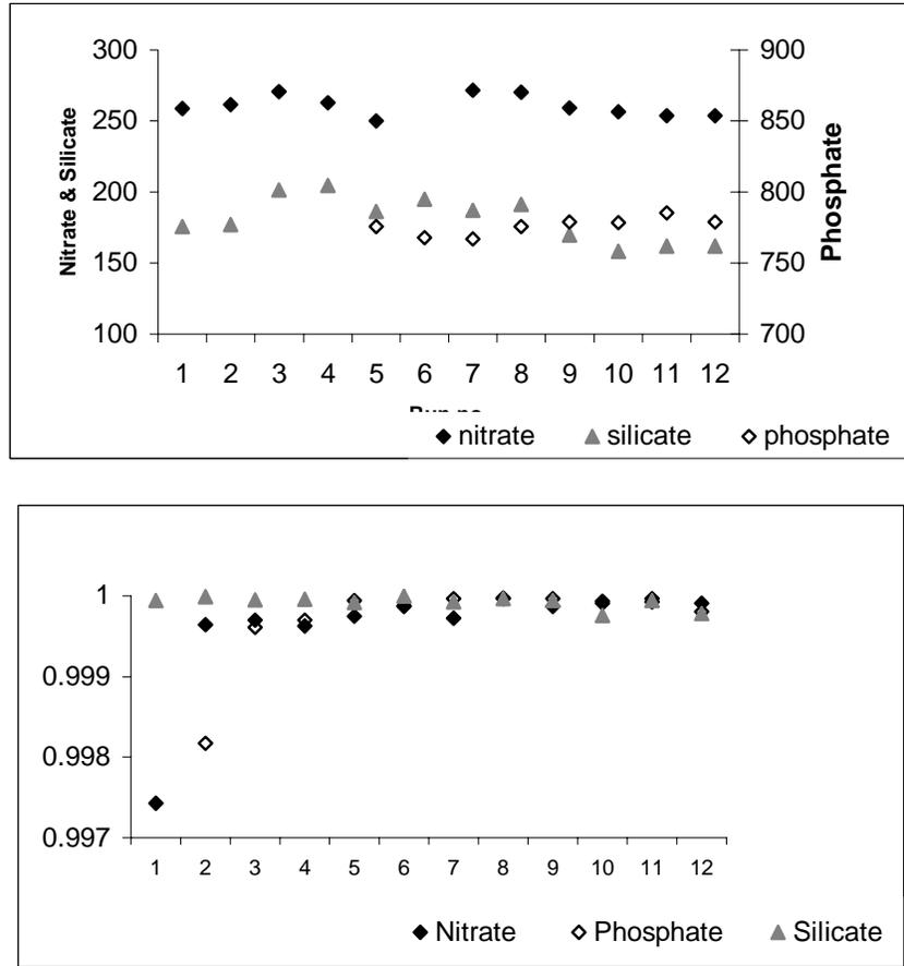
Fig 23. Upper graph, calibration constants, determined using the nutrient standard solutions, shown as a time series; lower graph, the goodness of fit for the calibrations.
