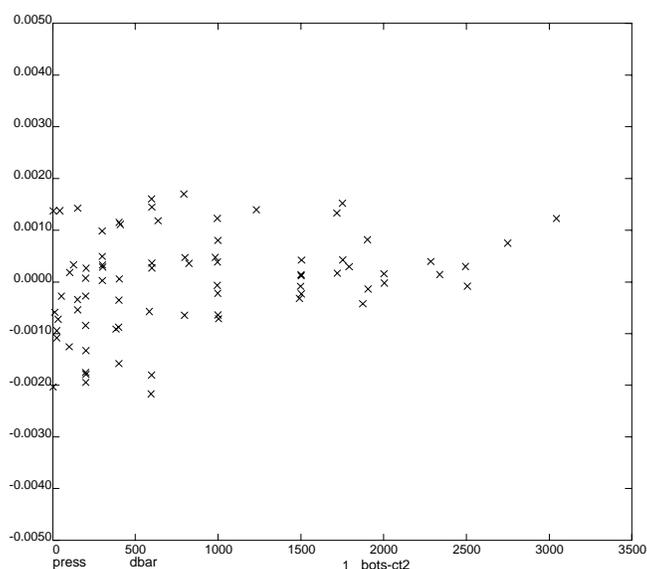
**Fig 10.** Final calibrated salinity residuals for the secondary sensor for stations 15071-15171.
