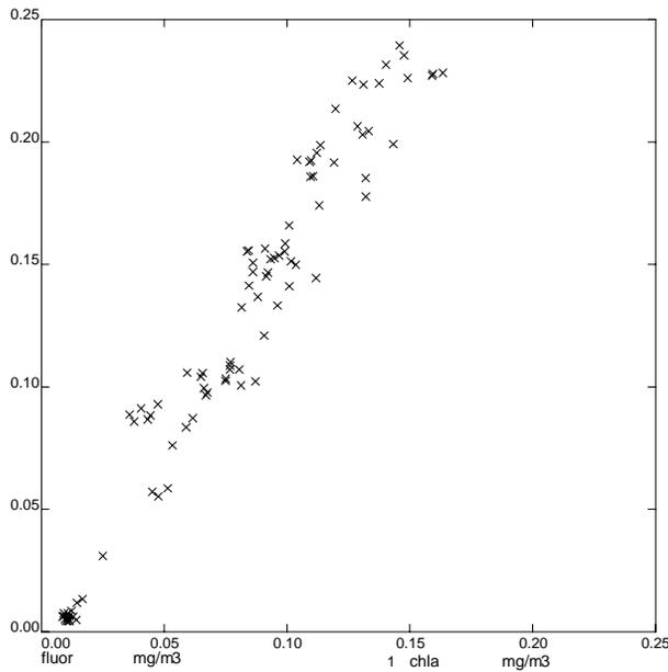
**Fig 12.** Chlorophyll from sample analysis versus CTD fluorescence derived value for stations 15071-15171.
