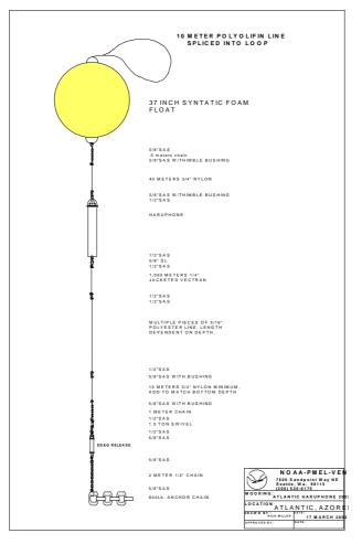
Figure III-2-1: Schematics of the hydrophone moorings deployed during the SIRENA experiment
