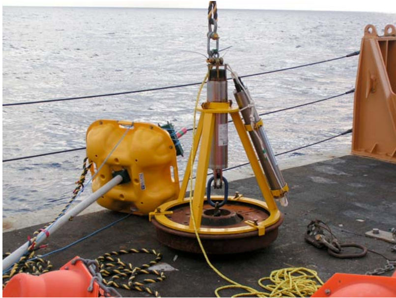
Photograph C.9: WBL4 tripod and buoy assembly
