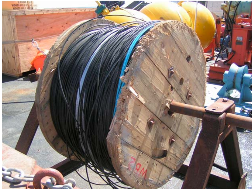
Photograph C.1: Damaged drum containing pre-wound wire for WB2
