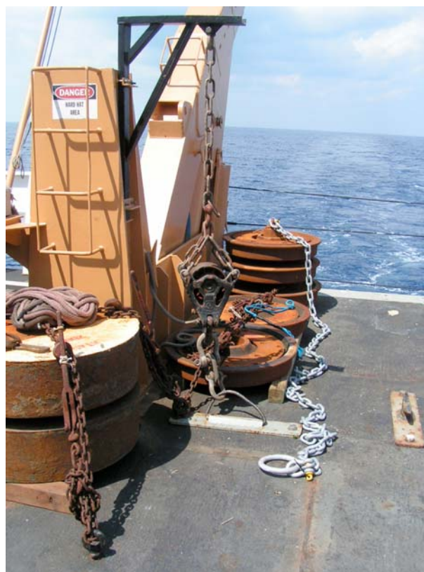
Photograph C.4: Diverter sheave on simple gantry. (RB0602)
