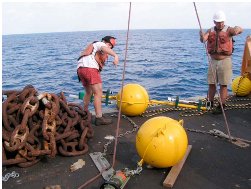
Photograph C.10: WB2 steel spheres – showing top buoy and 100m buoy.
