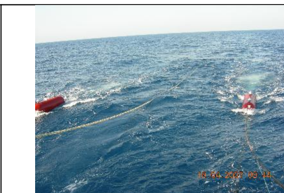
Fig. 2.3.1d: Airguns beams towed 14 m behind ship. Streamer is towed between the two beams.
