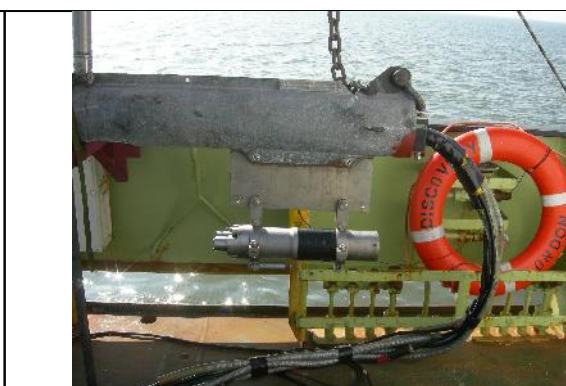
Fig. 2.3.1b : Detail of a mini GI airgun. The ombilicals include compressed air supply and electrical connectors (generator and injector solenoids, Time Break hydrophone).
