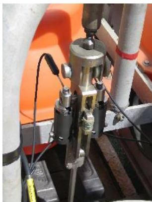
Figure 2.2.4: Titanium release and burn-wire mechanism
