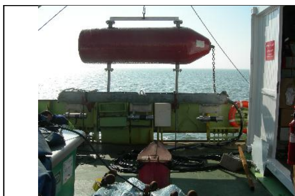
Fig. 2.3.1a : The seismic array includes 2 seismic beams (portside beam on the picture). Each seismic beam consists in 3 Soderia mini GI airguns, attached on a metallic frame hanging below the red floatation.
