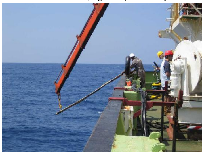
Figure 2.6.1. XBT deployment pipe on the starboard aft deck supported by knuckle crane.
