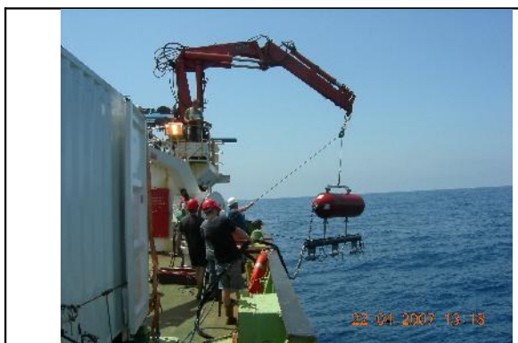
Fig. 2.3.1c : Deplyment/recovery of airgun beam on portside, using stern crane of RRS Discovery.
