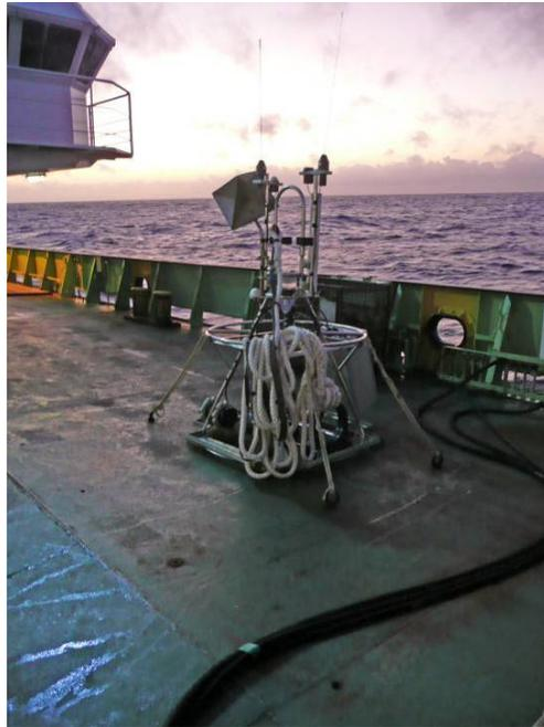
b – Telemetry Buoy Upper Tower Final Assembly
