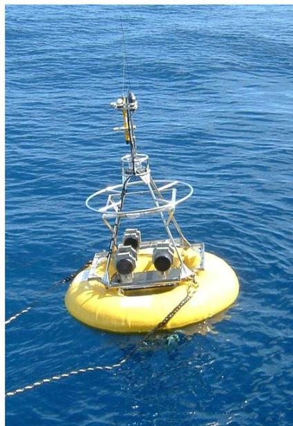
c – Telemetry Buoy Deployment
