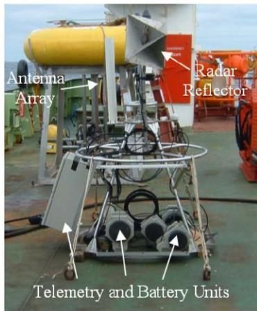
b – Telemetry buoy instrumentation tower
