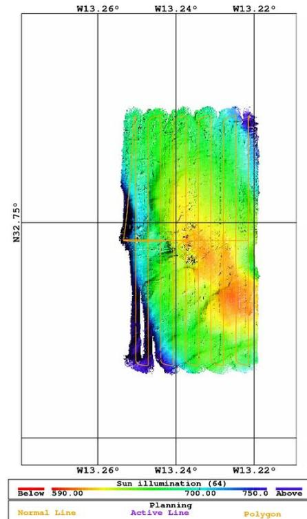
Figure 5. EM2000 multibeam survey data from the top of the Casablanca Seamount. Geothermal activity was identified at the summit (south west orange region).
