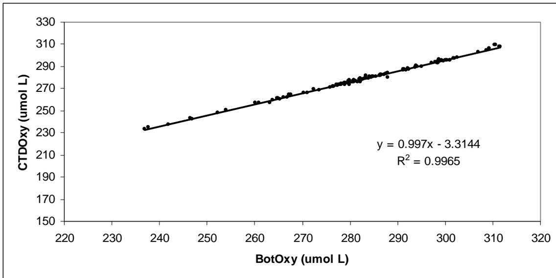
**Figure 5:** Bottle oxygen vs sensor oxygen concentrations. The fit is very good with an  $r^2$  of 0.9965. This plot was from the preliminary bottle oxygen data and also included all the outliers so this fit could be improved once quality controlling of the data is complete.
