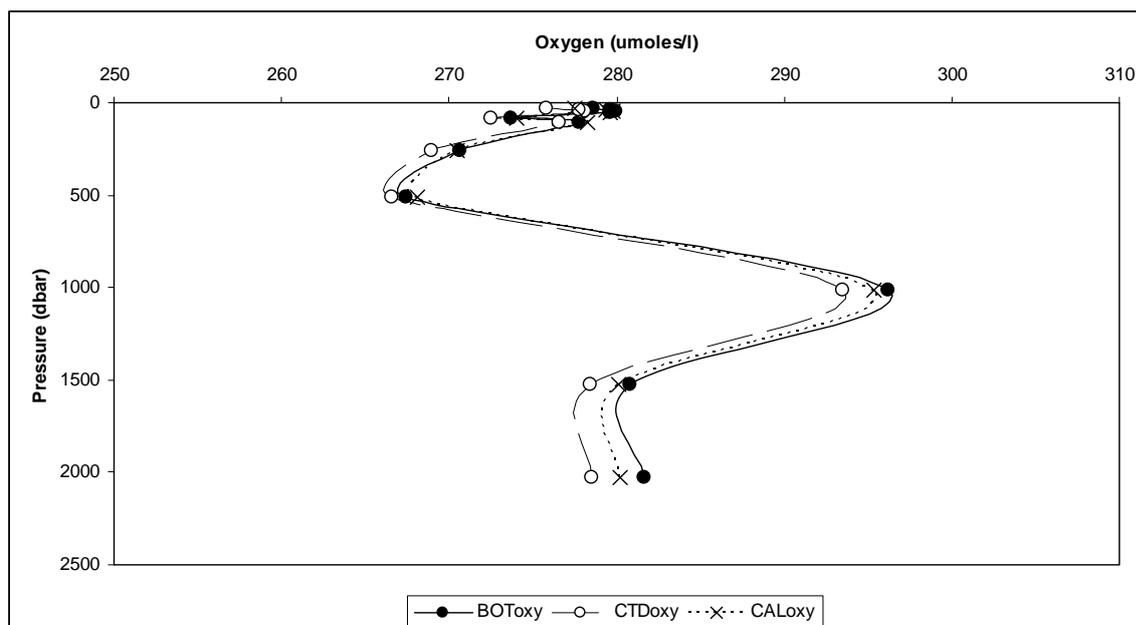
**Figure 6:** This profile from Station 20, CTDS023, shows the difference between the sensor oxygen value (CTDOxy) and the bottle oxygen derived from the Winkler titrations (BOToxy). Overlaid on this is the recalculation of the sensor oxygen (CALoxy) made using the regression from figure 5.
