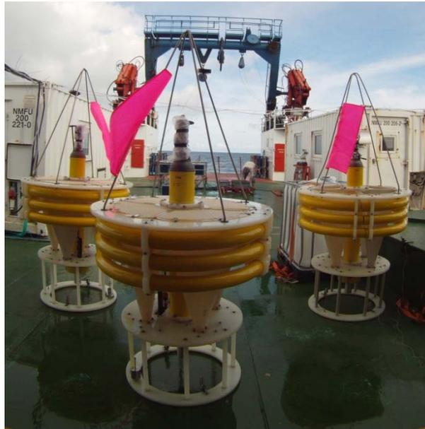
The Pelagra sediment traps have recently had modifications to upgrades which were added before the trails cruise JR221.
