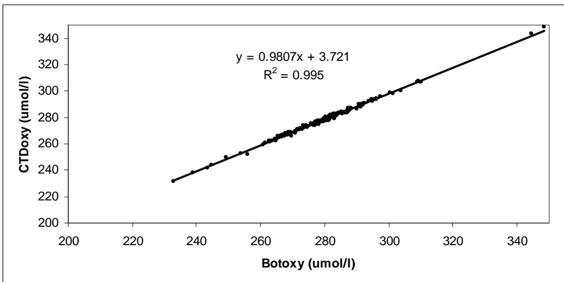
**Figure 4:** Bottle oxygen vs. sensor oxygen concentrations. The fit is very good with an  $r^2$  of 0.995.
