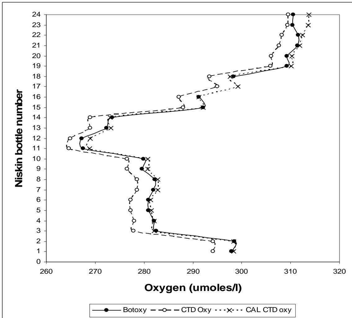
**Figure 7:** This profile from Station 4, Cast S006, shows the difference between the sensor oxygen value (CTD Oxy) and the bottle oxygen derived from the Winkler titrations (Botoxy). Overlaid on this is the recalculation of the sensor oxygen (CAL CTD oxy) made using the regression from figure 5. The sensor and bottle oxygen profiles now show a very good fit.
