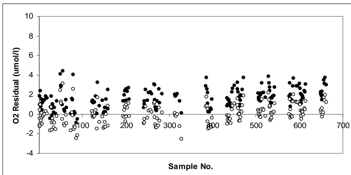
**Figure 5:** Residuals before and after the regression was applied. Closed circles are before the regression was applied. The mean residual for this group is approximately 2µmoles/l. After the regression (open circles) the mean residual is approximately 0.
