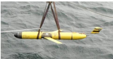
Unit 051 – Bellamite is a 1000m depth rated glider with a non-pumped Seabird CTD sensor
