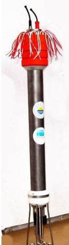
Figure 9.3: MSS90 microstructure profiler
