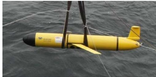
Unit 194 a 200m depth capable glider This science sensors are a pumped Seabird CTD, a WetLabs Triplet (CDOM, Chlorophyll-a and OBS Turbidity) and a Aanderaa dissolved oxygen Optode
