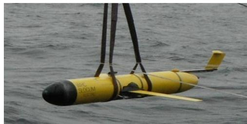
Unit 052 – Coprolite is a 1000m depth rated glider with a non-pumped Seabird CTD sensor
