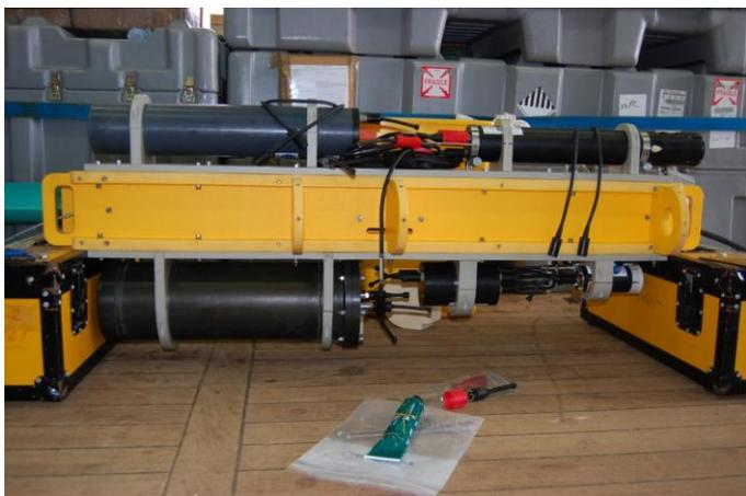
*Figure 10.1 Wirewalker setup (minus side buoyancy and guards)*
