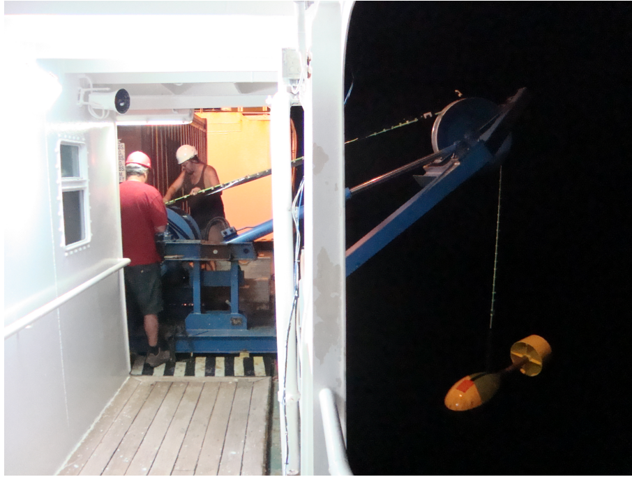
Figure 5: The FISH being deployed on the Port side.
