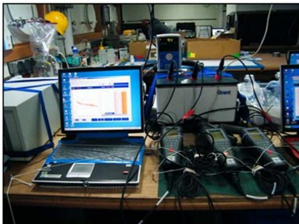
Figure 1. YSI PrODO optodes deployment and the water bath used.
