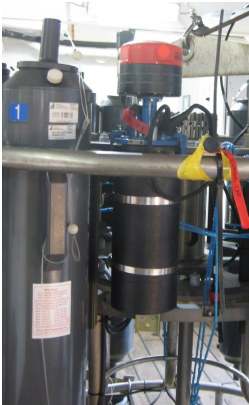
Figure 11: Pre-deployment calibration CTD with Seaguard in place of one of the 20 l Niskin bottles, please note the Turner Cyclops fluorometer mounted on the top bar facing out of the CTD rosette.
