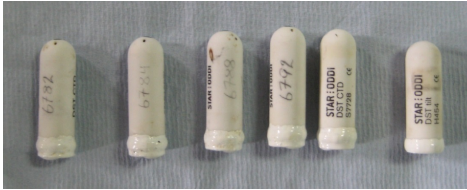
Figure 46: Image of the five recovered Staroddis; all have been removed from the fixings that bound them to the hose/frame and have been cleaned of any biofouling.
