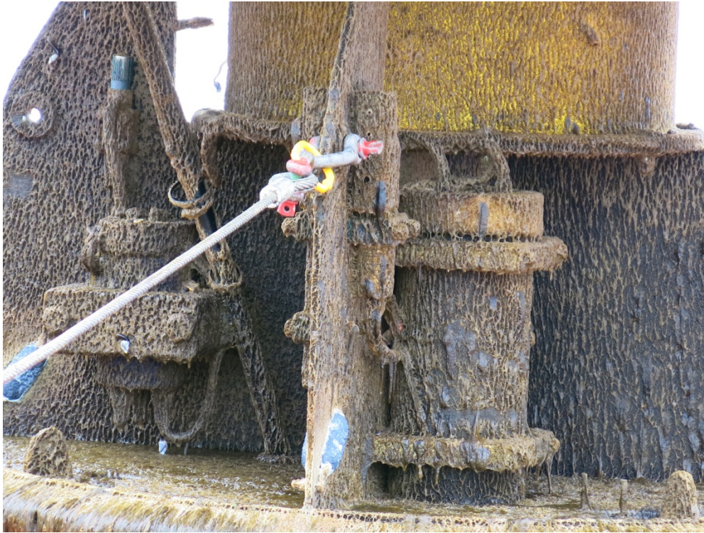
Figure 23: Picture of buoy keel after the recovery from deployment 2015-2016
