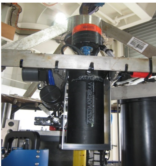
Figure 14: Seaguard mounted in PAP1 sensor frame before full integration of all sensors and harnessing.
