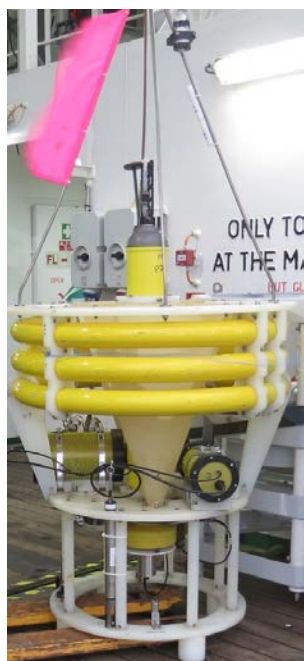
Figure 80: PELAGRA with the PELAGRA Cam mounted (the two green pressure housings). The left side pressure housing is for the camera and the right side pressure housing is for the flash gun.
