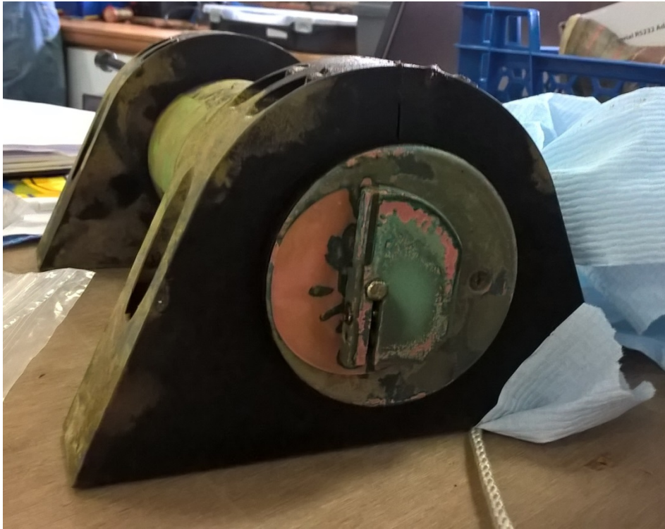
Figure 36: wetlabs s/n 3050 effective copper wiper
