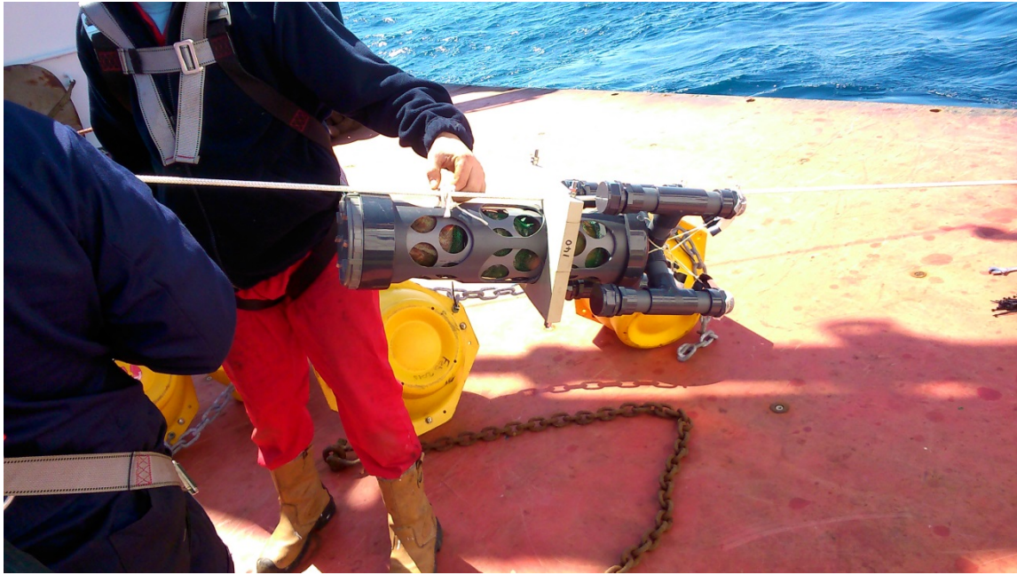
Figure 58: Colonisation traps with smaller larval settlement traps being attached to the PAP3 rope.
