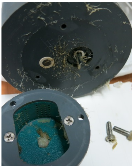
Figure 27: Biofouling on the sensor probe of SeaFET 257
