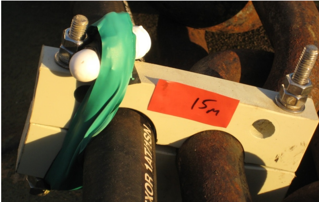
Figure 51: Staroddi secured on bracket along cable hose at 15 m mark.
