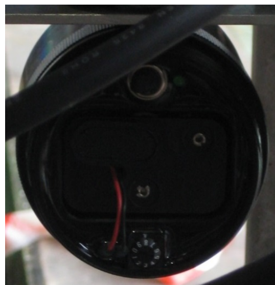
Figure 15: Image of ZebraTech wiper (taken before turning on) with back cover off showing position of timer
