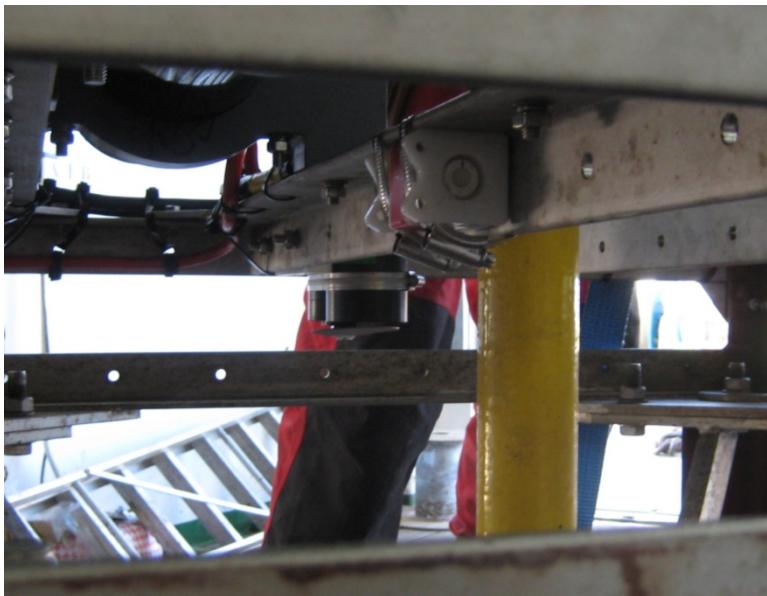
Figure 50: H454 being secured to cross bar of sensor frame before PAP1 deployment.
