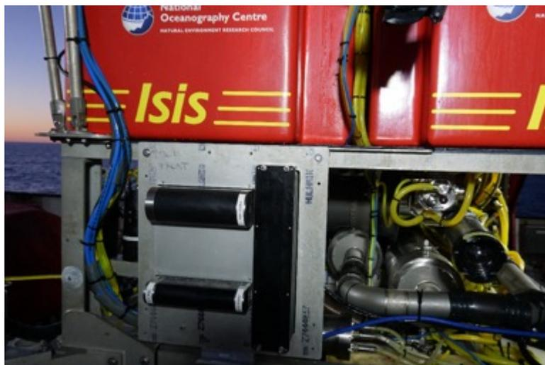
FIGURE 18: RESON 7125 TRANSDUCER SETUP ON ROV ISIS.
