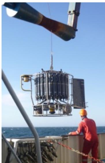
FIGURE 22: CTD DEPLOYMENT, SHOWING LADPCs AND OTHER SENSORS. PHOTO K.HENDRY.
