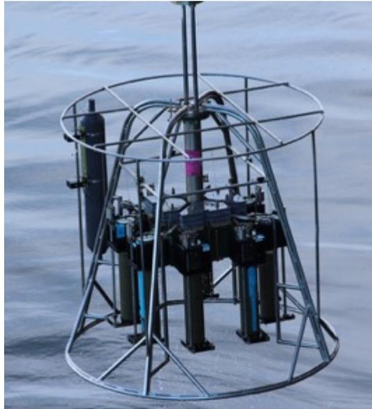
FIGURE 20: RECOVERY OF MEGACORE MGA04 ON JULY 24TH. ALL EIGHT CORES CONTAINED SEDIMENT AND THE SEDIMENT-WATER INTERFACE: HALF OF THE TUBES WERE DRILLED FOR POREFLUID SAMPLING, AND TAPED UP FOR DEPLOYMENT. PHOTO BY M. BADGER.
