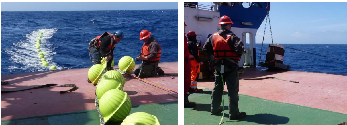
Figure 8 – Glass balls (left) and anchor (right) deployment
