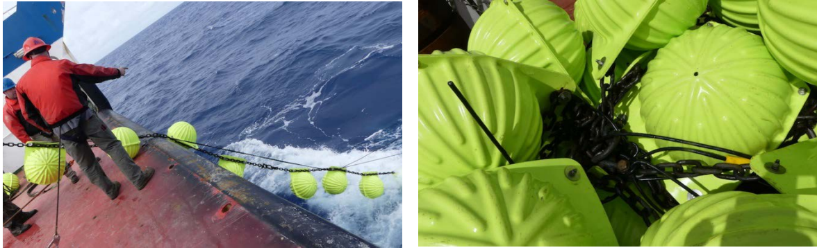
Figure 13 – Wire rope draped over the 2nd set of balls, and wuzzled in the last cluster.
