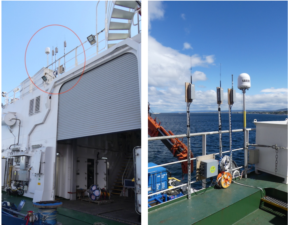
Figure 4 – OOI Telemetry positioning on aft Boat Deck rail
