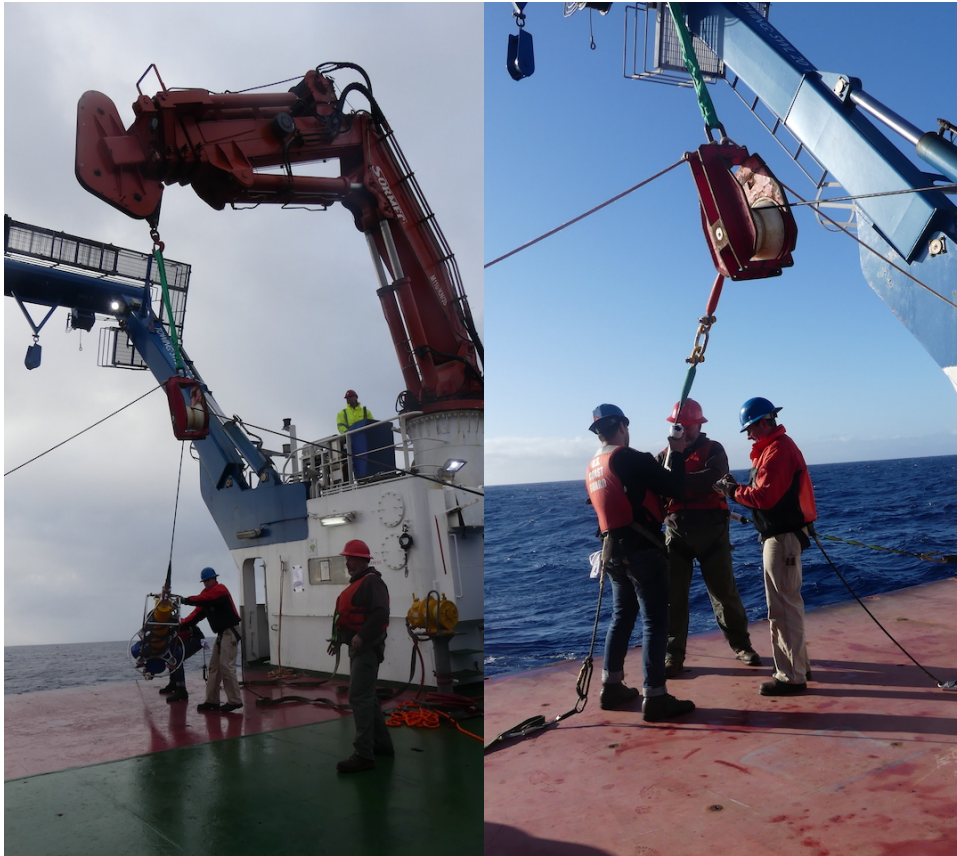
Figure 6 – Deployment of ADCP cage (left), and attaching instruments to the wire rope (right).
