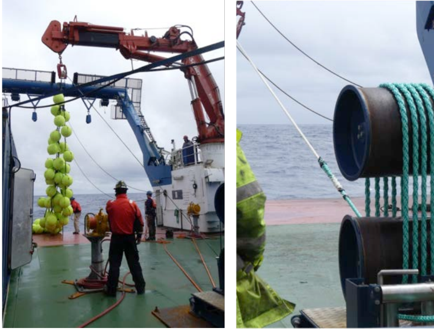
Figure 9 – SUMO-3 glass balls (left) and synthetic rope (right) being hauled in.
