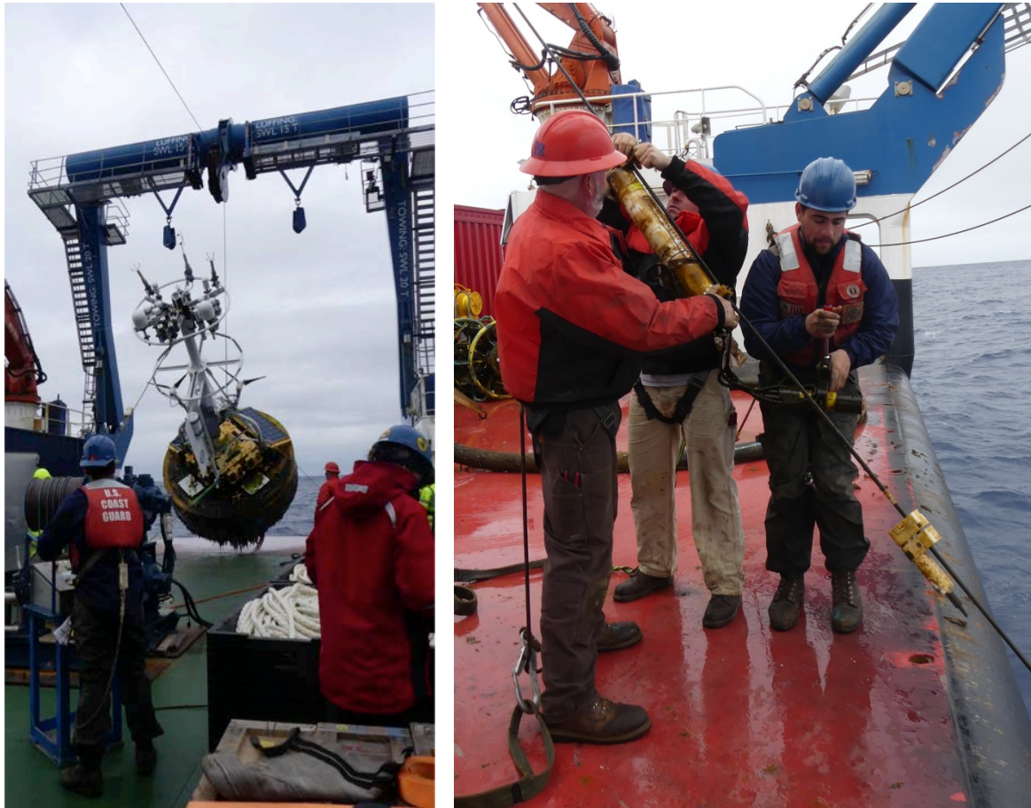
Figure 11 – Recovery of the SUMO-3 surface buoy (left), and removal of instrumentation clamped on the wire rope (right).
