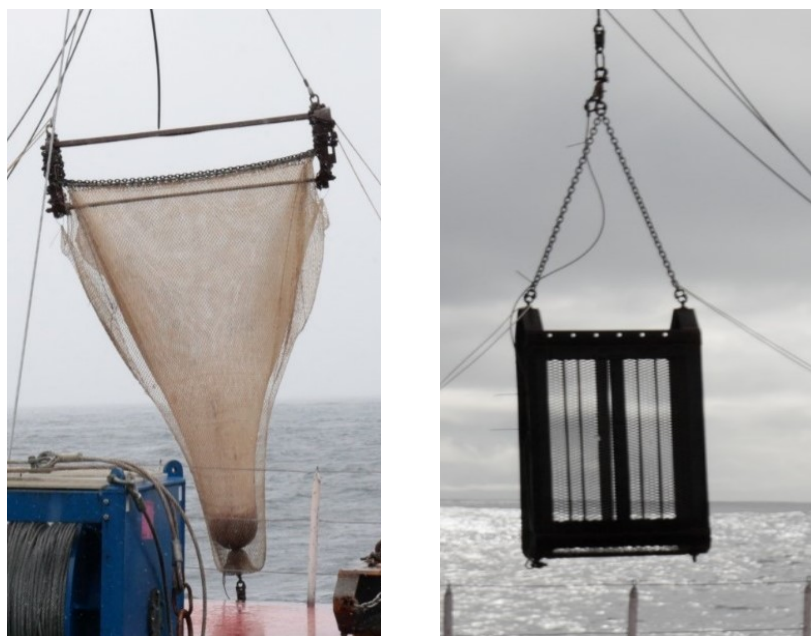
Figure 5.6. Recovery of the Agassiz trawl (left) and dredge (right) from the aft deck of the RRS Discovery during DY99 showing the bridles, weak links and recovery bridle (dredge).
