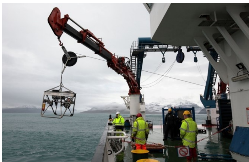
Figure 5.4. Trial deployment of the deep-water video and still camera system from the RRS Discovery .
