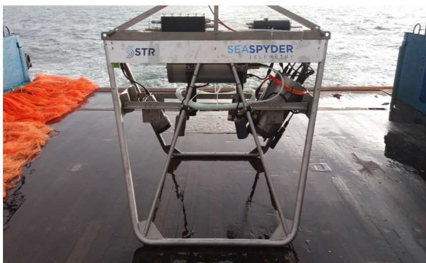
Figure 5.3. The deep-water video and still camera system deployed during DY99. The still and video camera system and laser pointers are mounted on the right with the flash system on the left.
