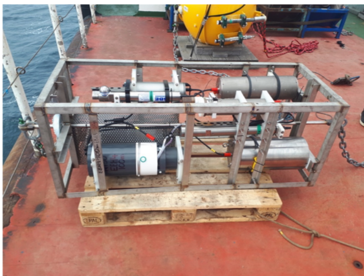
Figure 26: BGC sensor frame ready to be deployed @50m on EBH3 (ignore incorrect labelling on sensor as moved from not-deployed EBH4). Sensors comprise one OTE-Nitrate sensor (dark grey plastic) with associated battery case (bottom right) and shielded waste receiver (grilled square box behind sensor), SeapHOx sensor (top left), Contros pCO2 sensor (top front) and associated battery pack (back right) and MicroCAT (front middle of frame).
