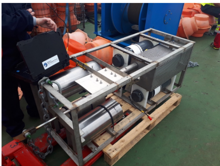
Figure 27: BGC sensor frame being prepared for deployment @400m on EBH3. Sensors comprise 2 OTE sensors (dark grey plastic) with two associated battery cases (left) and shared waste receiver (grilled square box top right), Contros pCO2 sensor and battery pack (both obscured in this picture) and two MicroCATs – one with oxygen (clamped underneath the white square).
