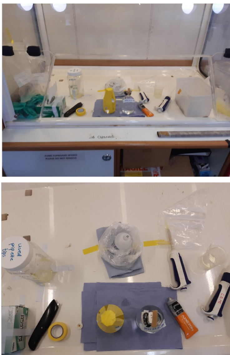
Figure 22: Photographs of the fume hood set-up and examples of how bottles were sealed with tape (left bottle) and clip and band (right bottle).
