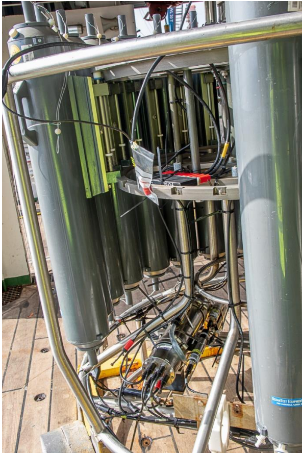
Figure 3.9: Installation of Oceanids Hub on CTD frame, taking power from CTD SBE-9Plus
