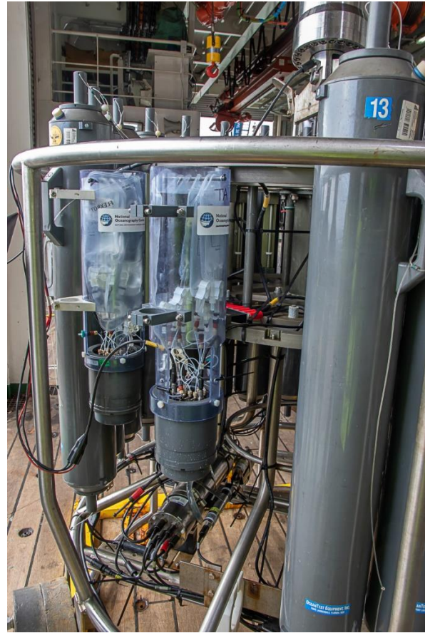
Figure 3.10: From the Oceanids Hub individual cables run to the two Wet Chemical sensors
