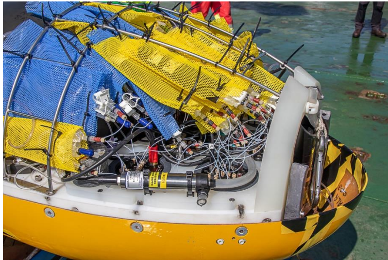
Figure 3.1: AutoNutS sensors showing reagent bags and manifold pump/outlet
