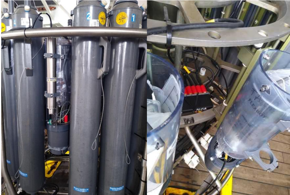
Figure 5.3: On the left, sensors battery powered, on the right, sensors powered from the Oceanids hub.
