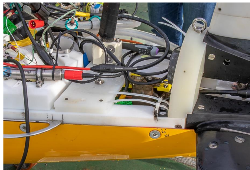
Figure 3.6: STAFES outlet hose position (2 cable ties to rear)
