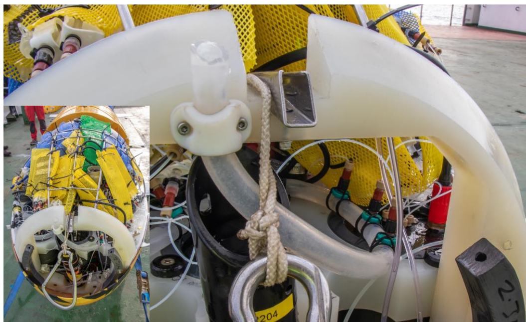
Figure 5.2: Sampling manifold for Autonuts. Inlet is in the top centre and SBE-5T pump and outlet is to the left of the image. Insert: Installation of Autonuts sensors in front of ALR.
