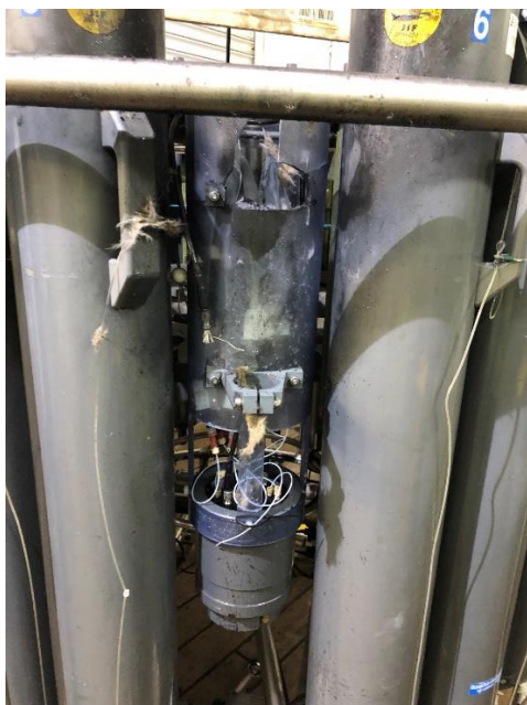
Pictures show the damaged nitrate sensor after the incident along with damage to CTD frame and water sampler
