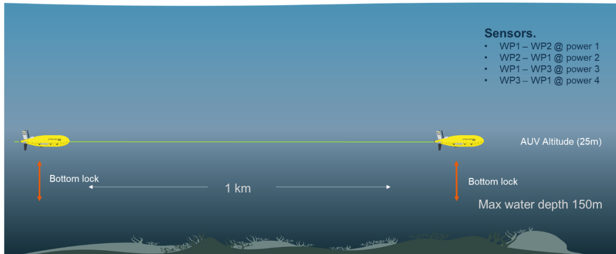
Figure 2.4: ALR power runs with sensors also switched on.
