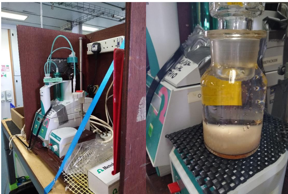
Figure 5.11: Winkler titration set up (794 Basic Titrino, Metrohm) and an oxygen sample after collection.
