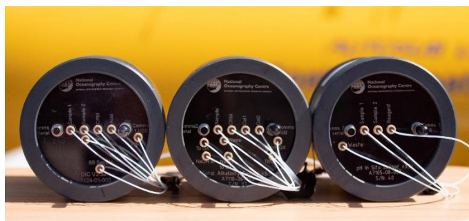
Figure 6.1: The tree LOC sensor for the measurements of pH, TA and DIC
