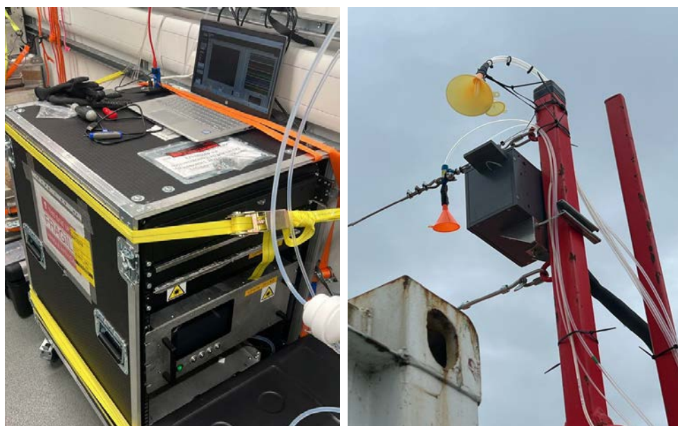
Figure 18. Photographs of the LIF-SO 2 instrument in the rack (left) and the SO 2 inlet on the roof of the BAS container (right), covered by an orange funnel (marked with an arrow).
