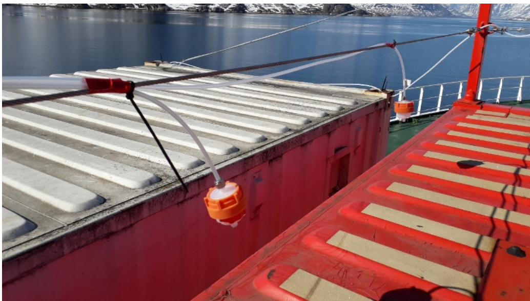
Figure 20: Photo of the filter cassettes on the roof of the lab container.
