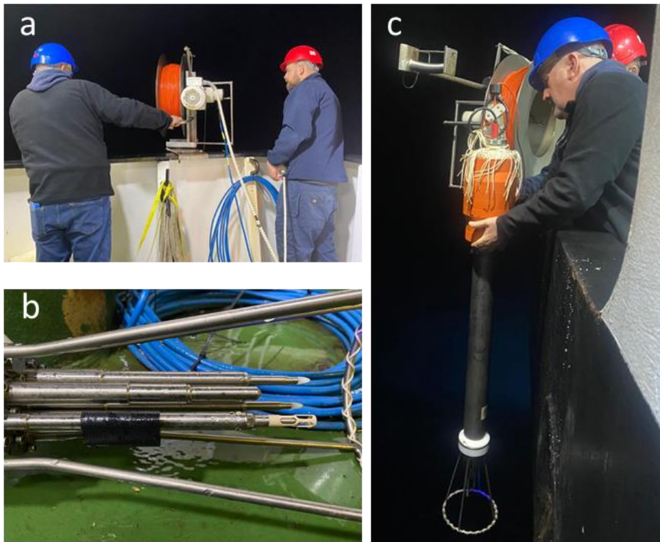
Figure 1 Deployment of MSS 90. a- winch operation b- deployment of MSS90. c – sensors of MSS90
