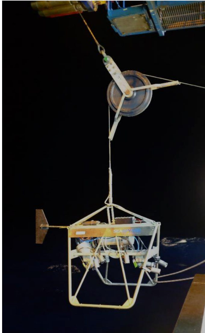
Figure 30 – Deployment of the towed camera.
