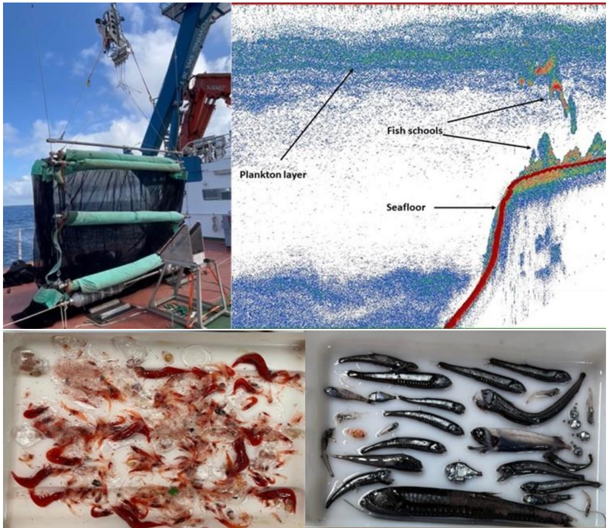
Figure 20 – The Rectangular Mid-water Trawl (RMT) while being tested on the deck of RRS Discovery. Adjacent to this is an annotated echogram illustrating the different layers that were targeted using the RMT and the final two images depict a representative catch from the RMT.
