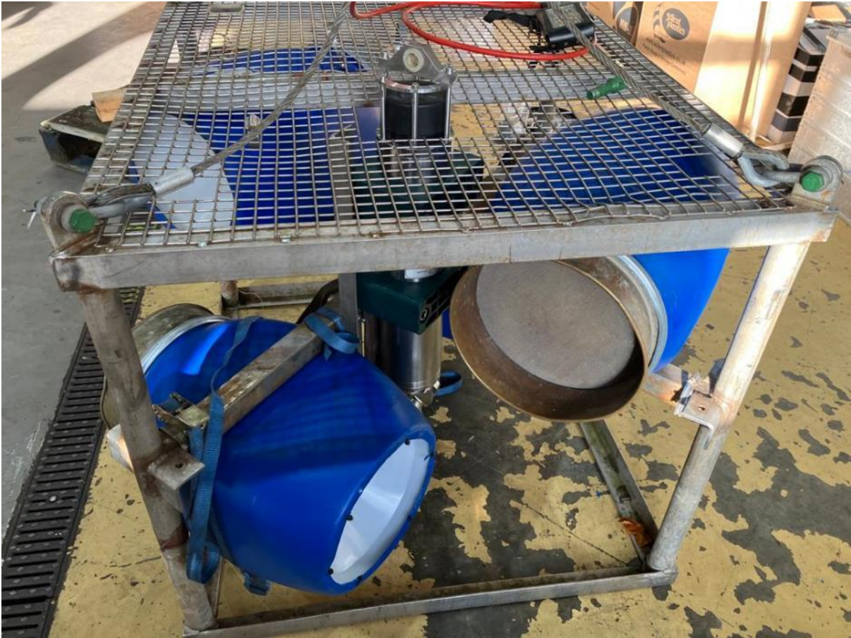
Figure 42 – The baited amphipod trap showing the acoustic release in the centre and perpendicularly mounted benthic and suprabenthic cylinders.
