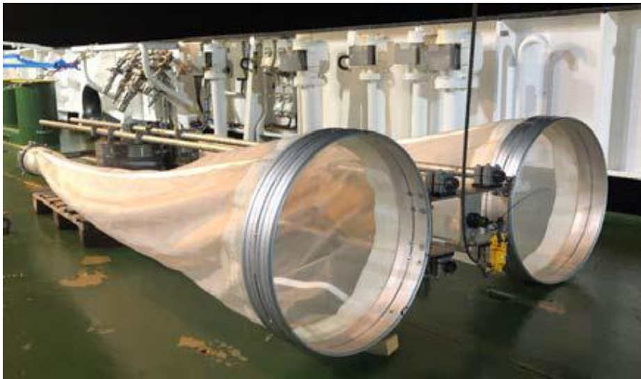
Figure 50 – Motion compensated Bongo nets with 100 \mu\text{m} and 200 \mu\text{m} mesh size nets and cod ends.
