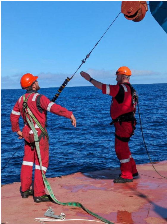
Figure 2: (a) Dissolution sample tubes attached to the mooring line. (b) Sample tubes on their way to getting rinsed.
