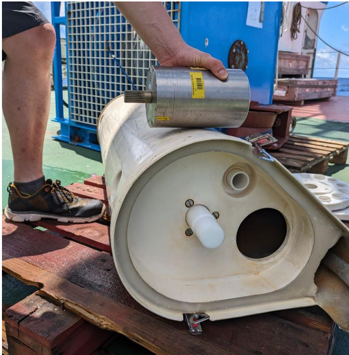
Figure 3: Recreation of how the sediment trap motor was found inside the sediment trap, instead of being placed in the hole on the right of the trap.
