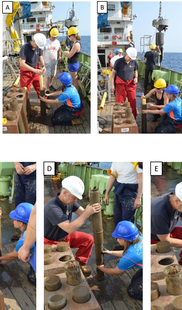
Figure 7.3. Photos demonstrating taking sub-cores using the trigger weight core liner. A) The core liner is slowly pushed into the centre of the multi-core. B) A cap is placed on the top of the core and labelled as the top of the core. C) The multi-core and core liner have carefully been turned upside down and the bung is removed. D/E) The core liner is held securely upright, and the multi-core is pulled up.
