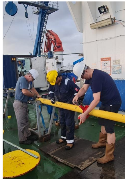
Figure 8.9: Labelling the PVC liner with the system mentioned below and cutting the liner into 1.5m sections with a core cutter.
