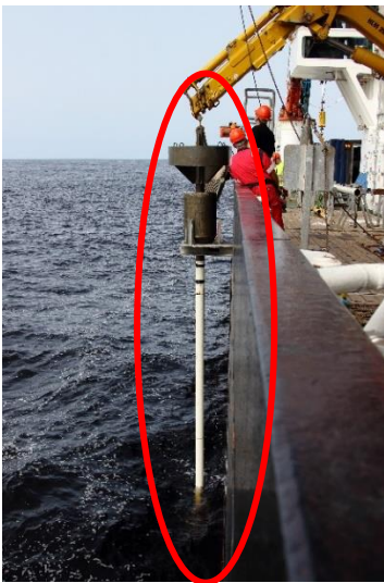
Figure 8.3: Once trigger core has been removed (fig.2) then piston core (red circle) is placed on a stand using two cranes working simultaneously.
