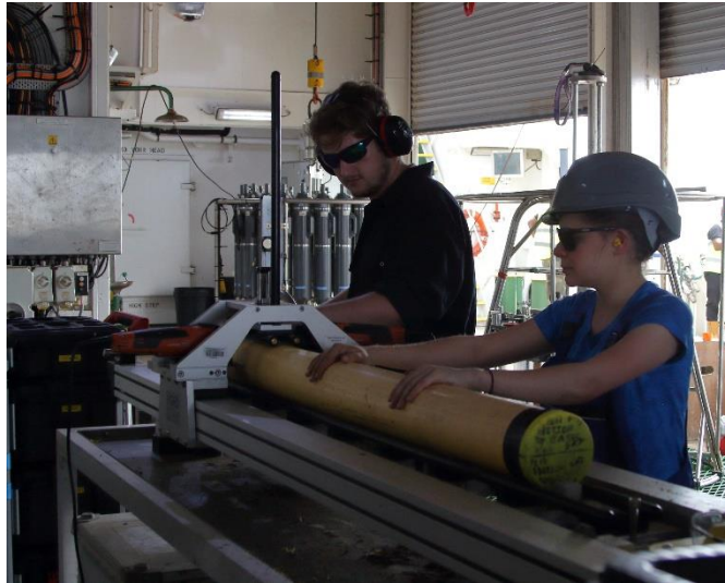
Figure 8.10. Sediment core splitting using a core splitter.
