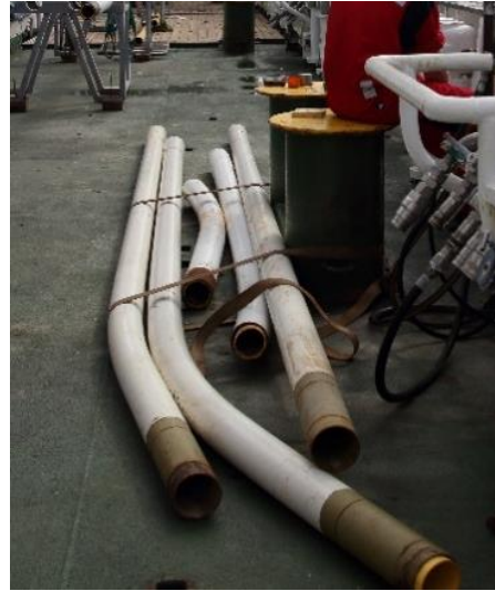
Figure 8.7: On some occasions where the freefall calculations and the sediment were too rigorous, the barrels will have bent to the 1500kg weight attached at the top.
