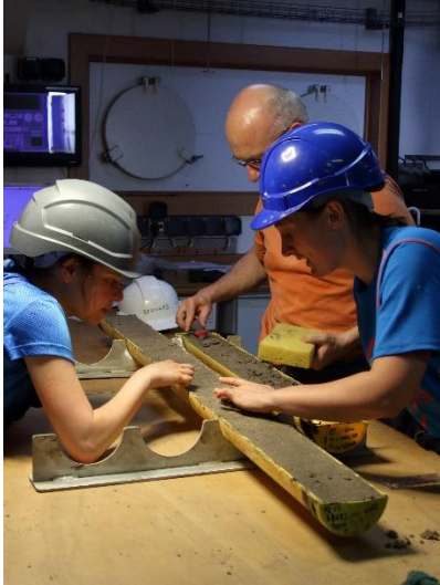
Figure 8.11. Sediment record cleaning and initial scientific curiosity in the sediment grain sizes.
