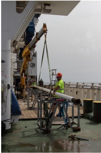
Figure 8.6: The barrel is then placed on stands where the PVC liner will be removed and split into 1.5m sections for processing.
