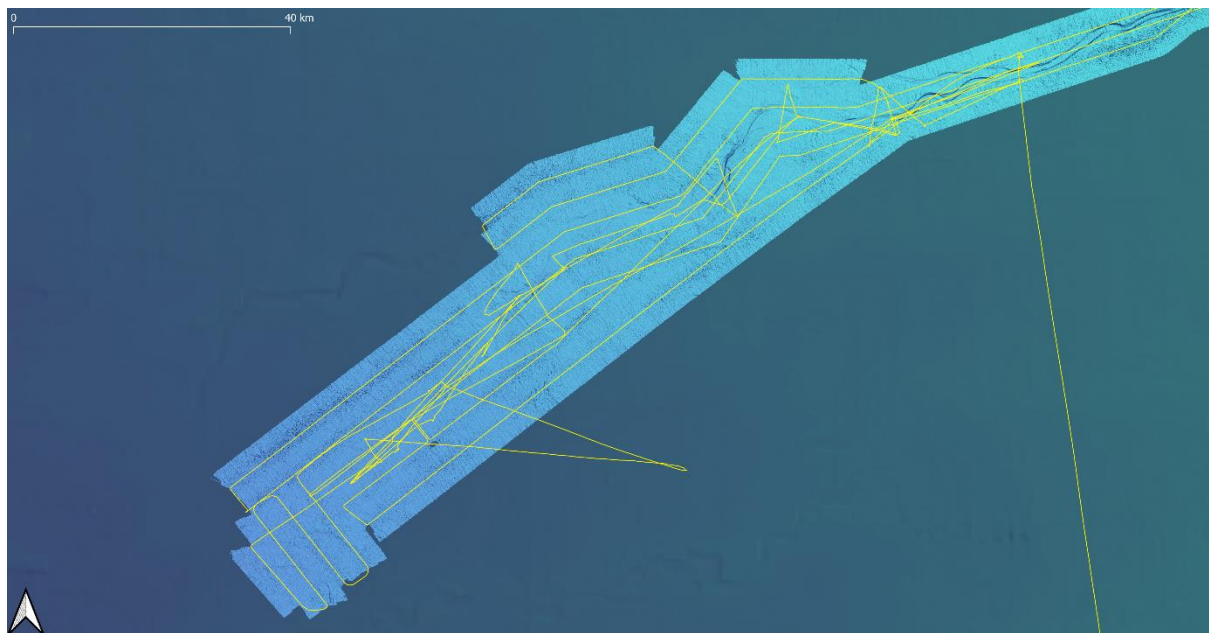
Figure 1.2. Map of the lobe area, showing the ship track lines and swath multibeam data collected.
