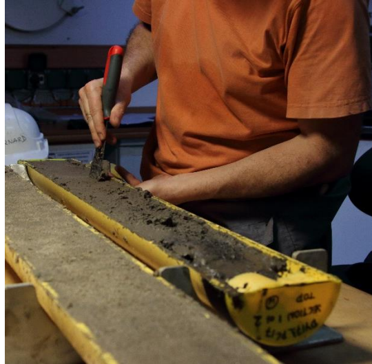
Figure 8.12. Cleaning excess sediments before the sediment record analysis.
