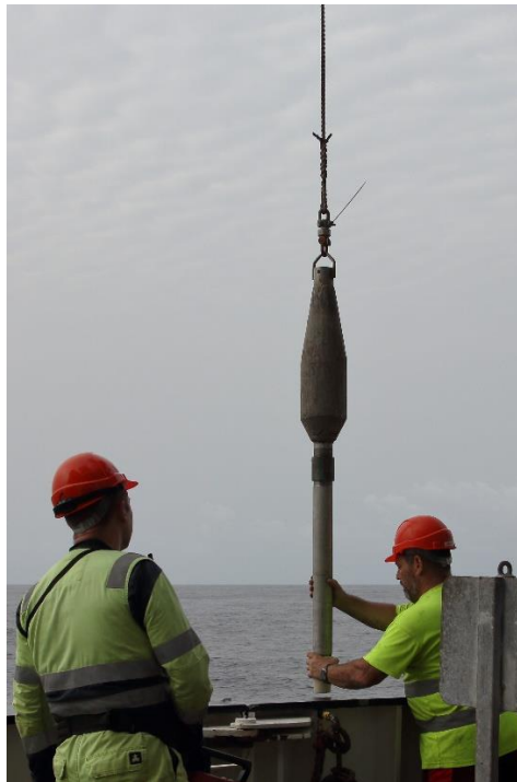
Figure 8.2: Image taken from the DY173 cruise, before attachment to the barrel of the piston core.
