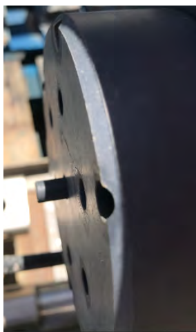
Figure 12.6 Pressure pin protruding from TA 20 on recovery, indicating seawater inside the sensor housing.
