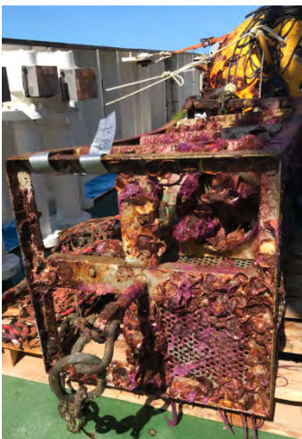
Figure 12.2 Biofouling on the 50 m EBH3 frame.
