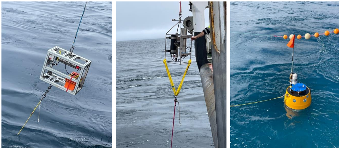
Left: Drift-CAM; middle: RESPIRE trap; right: surface buoy with light, flag and GPS tracker and AIS.
