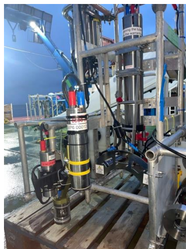
Red Camera Frame with both UVP5 (as standard) and UVP6 for cross-sensor calibration and validation
