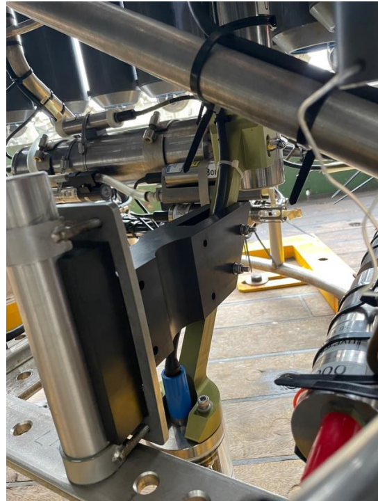
UVP6 and external battery fitted onto the CTD rosette using a custom made adapter for the CTD kit supplied by LOV
