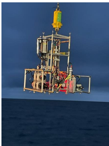
Red Camera Frame with both UVP5 (as standard) and UVP6 for cross-sensor calibration and validation
