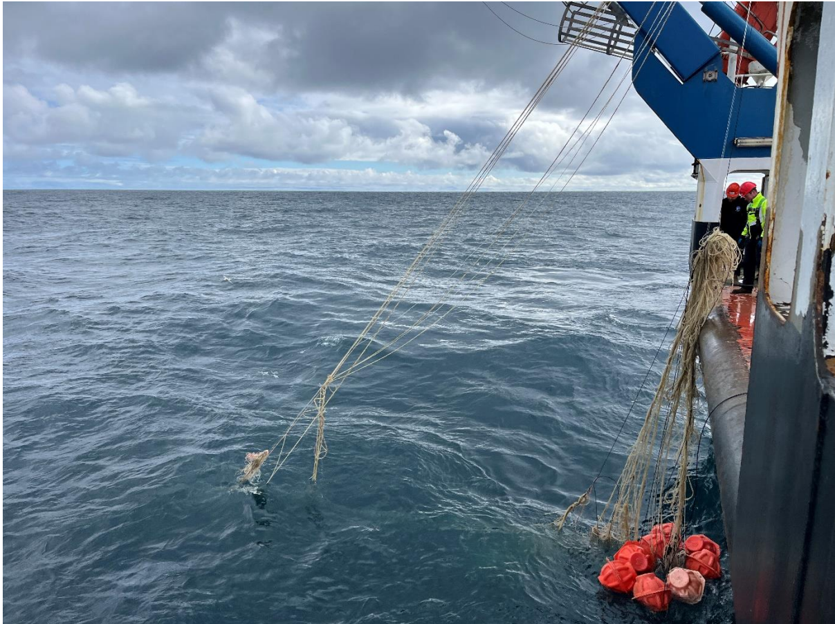
Figure 30: IB3 recovery with fishing line tangled along the mooring.
