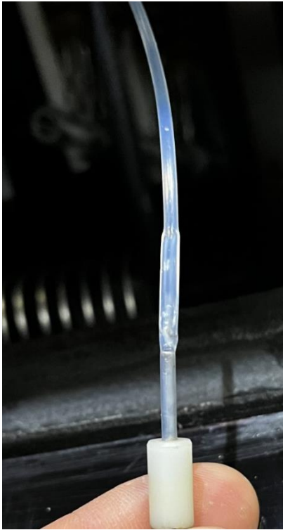
Figure 2: Kinked tubing at conductivity cell inlet.
