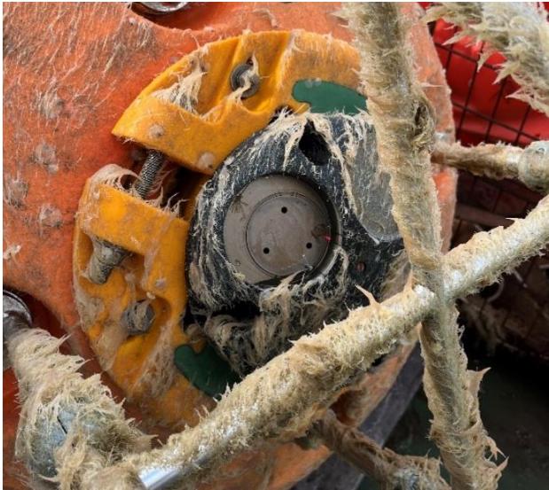
Figure 39: Missing transducer head on ADCP S/N 20957
