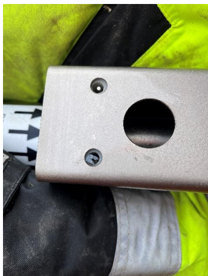
Figure 31: Obstructed exhaust of Microcat.
