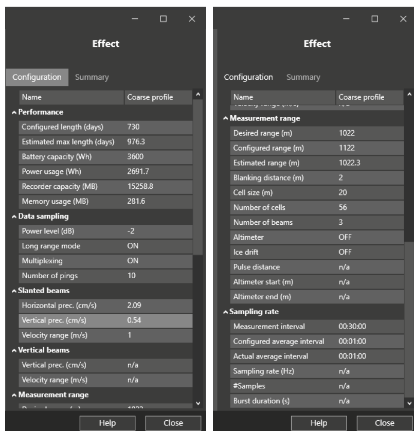
Figure 44: Configuration parameters for DY181 deployment of RHADCP, Nortek S55 sn J20268-002
