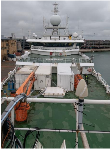
Figure 3: View from the foremast towards the ship's bridge. Showing the containers with the majority of the atmospheric instrumentation and the inlet sampling tubing which can be seen running from the rail of the foremast to the port side of the middle container.
