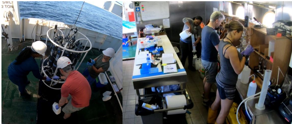
Figure 11: Pictures illustrating the collection of seawater from the CTD and the filtration in the laboratory before preservation
