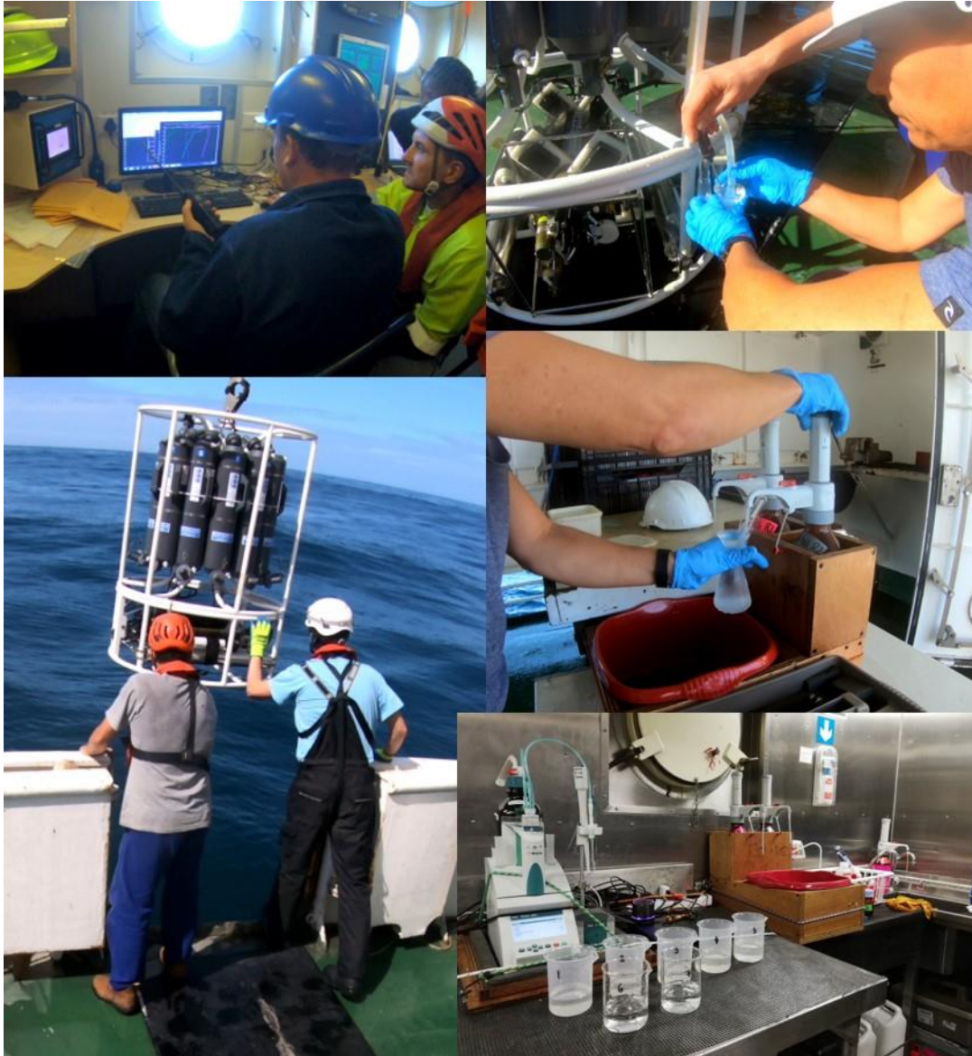
Figure 4: Pictures showing the CTD deployment and collection of dissolved oxygen samples for CTD calibration
