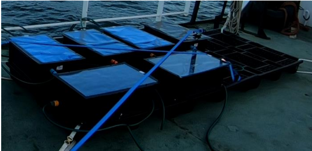
Figure 12: Pictures of the incubation boxes on the deck with the different light intensity level
