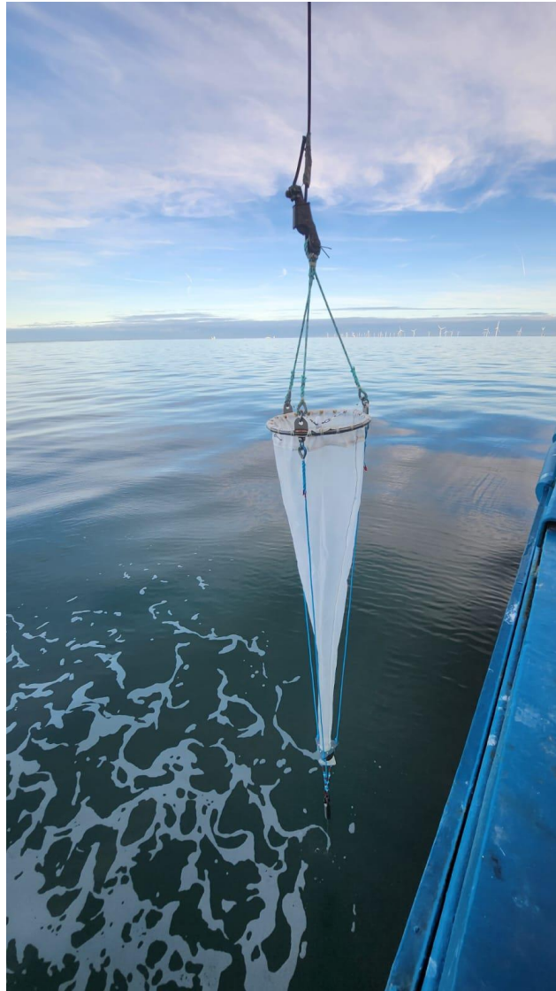
Figure 11: Plankton ring net being deployed off the side gantry at Liverpool Smart buoy station.
