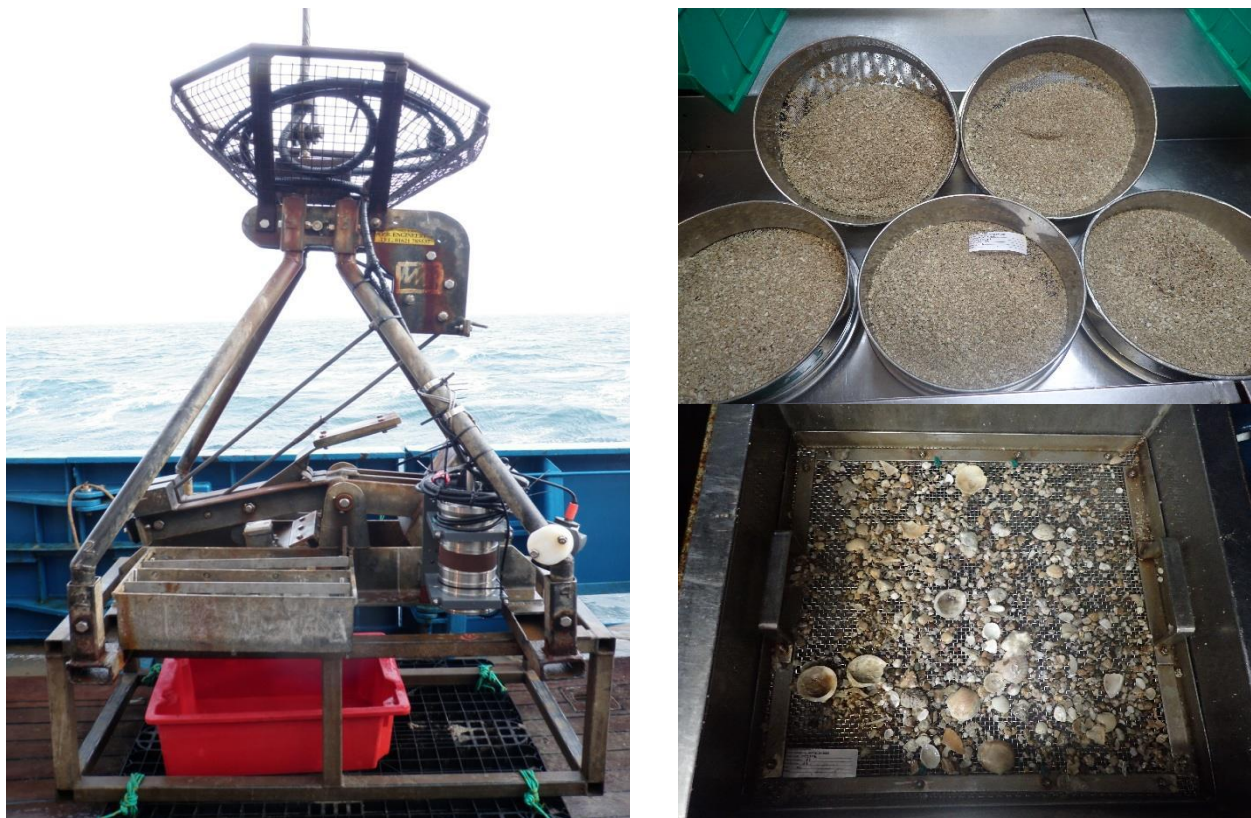
Figure 4 The mini-Mini-Hamon grab sampler plus the 1mm and 5mm sieved sample from a typical sampling location
