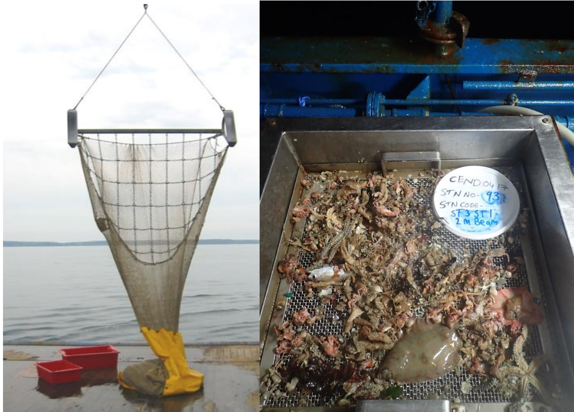
Figure 6 - A 2m Jennings's beam trawl with a typical catch ready for sieving.
