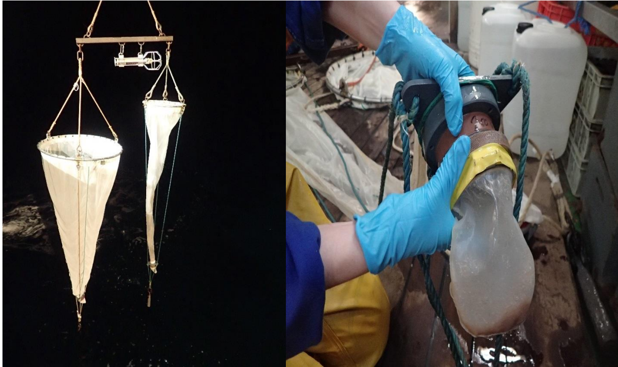
Figure 3 - Deployment of the two plankton 'ring' nets and the resulting plankton sample
