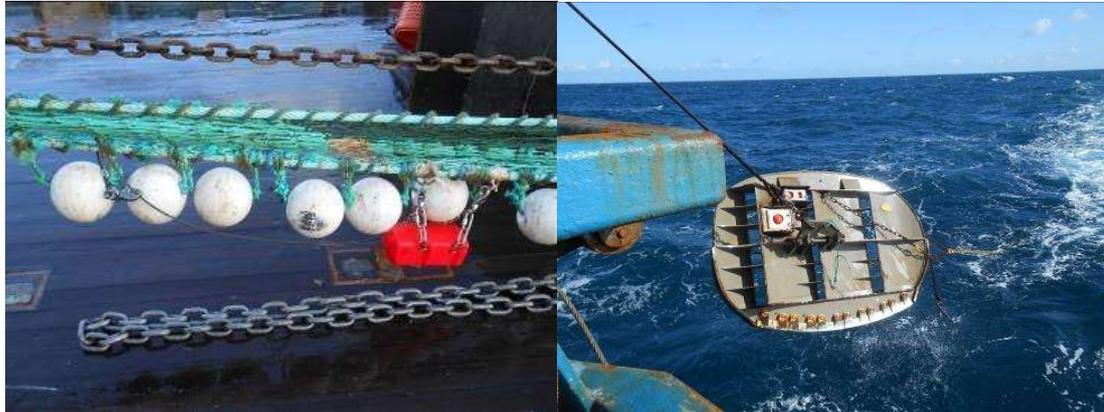
**Figure 5:** Trawl showing (left) Scanmar wing end sensor and (right) starboard door with Scanmar door sensor in door pocket
