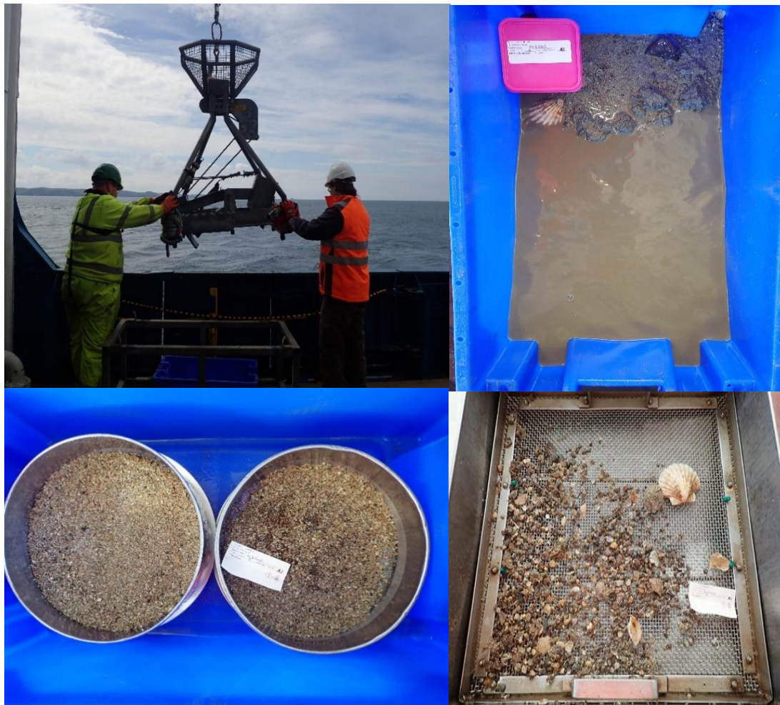
Figure 6: The mini-Hamon grab sampler plus a typical retrieved sample along with 5mm and 1mm sieved samples
