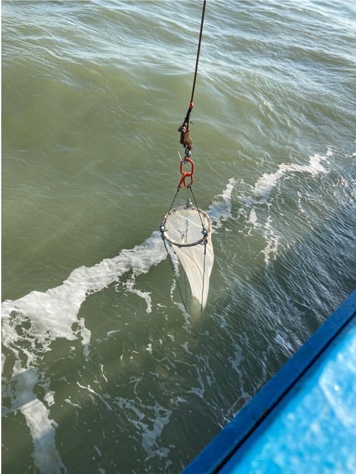
Figure 7. Zooplankton ring net (0.5 m, 200 \mu m mesh) deployment.
