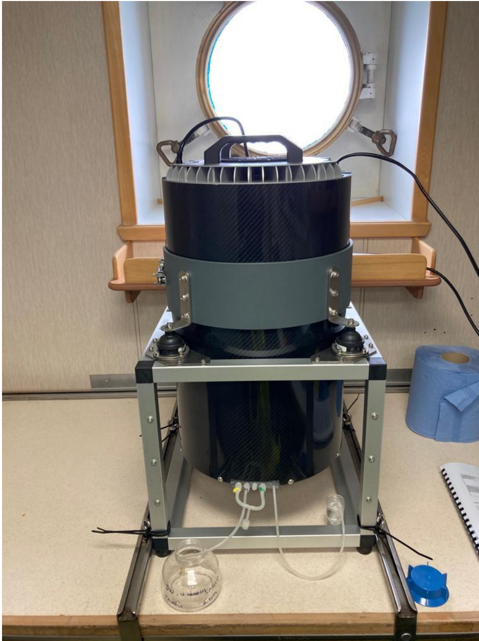
Figure 2. Flow cytometer sampling phytoplankton from a discrete water sample.
