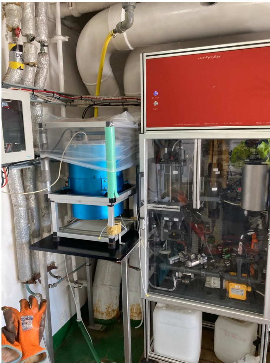
Figure 1. Flow cytometer installed and connected to the FerryBox on board the RV Cefas Endeavour.
