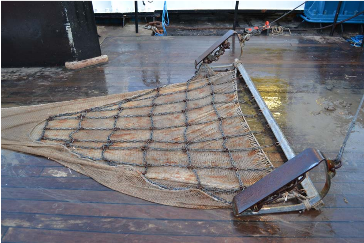
Figure 2 - 2m Jennings beam, showing the chain matt and the extra chain on the shoes and around the foot-rope. Photo by Robin Masefield (Cefas).
