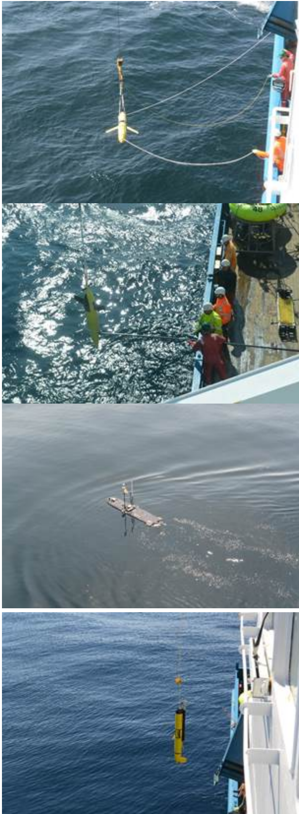
Figure 2. Clockwise from top left corner: deployment of NOC Slocum Glider, recovery of UEA seaglider, recovery of NOC Slocum Glider and deployment of Cefas Wave Glider Lyra.
