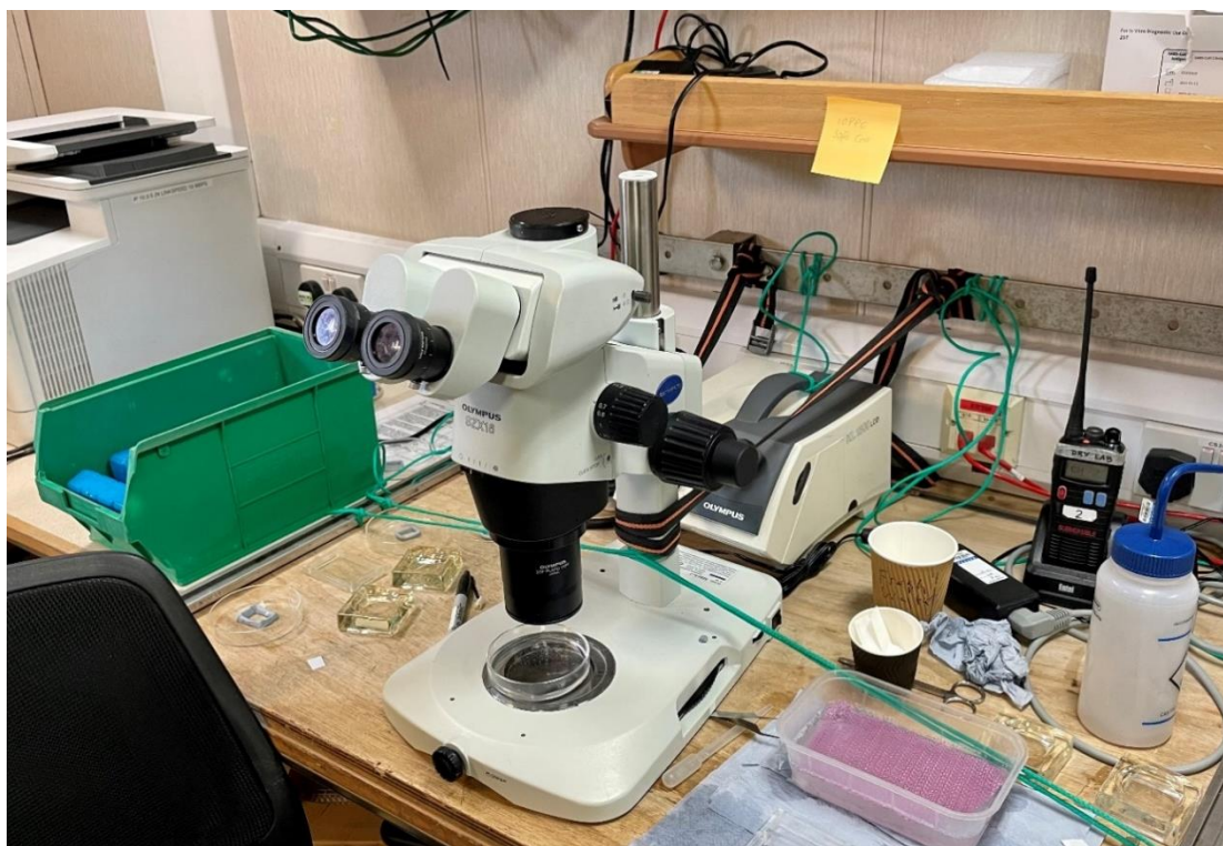
Figure 7. Stereo microscope and reflected top and bottom light used to identify and remove all ichthyoplankton eggs and larvae from samples.
