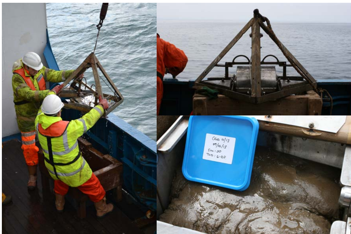
Figure 4 – Use of the 0.1 m 2 Day grab during retrieving. Photo by Robin Masefield (Cefas).
