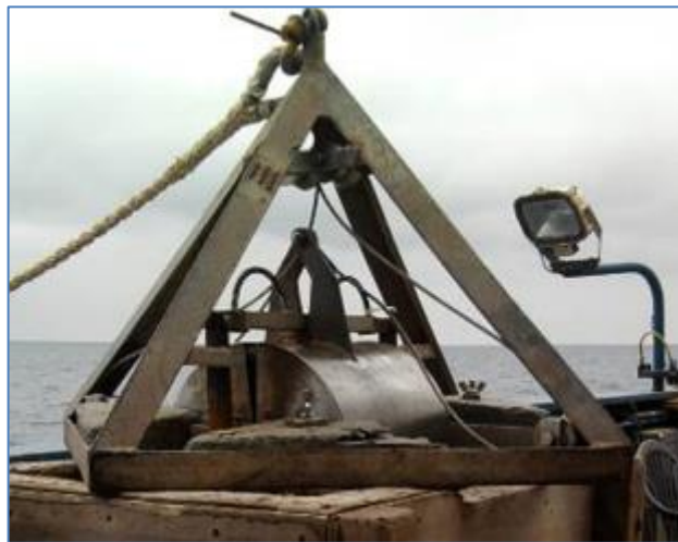
Day grab used to collect sediment samples
