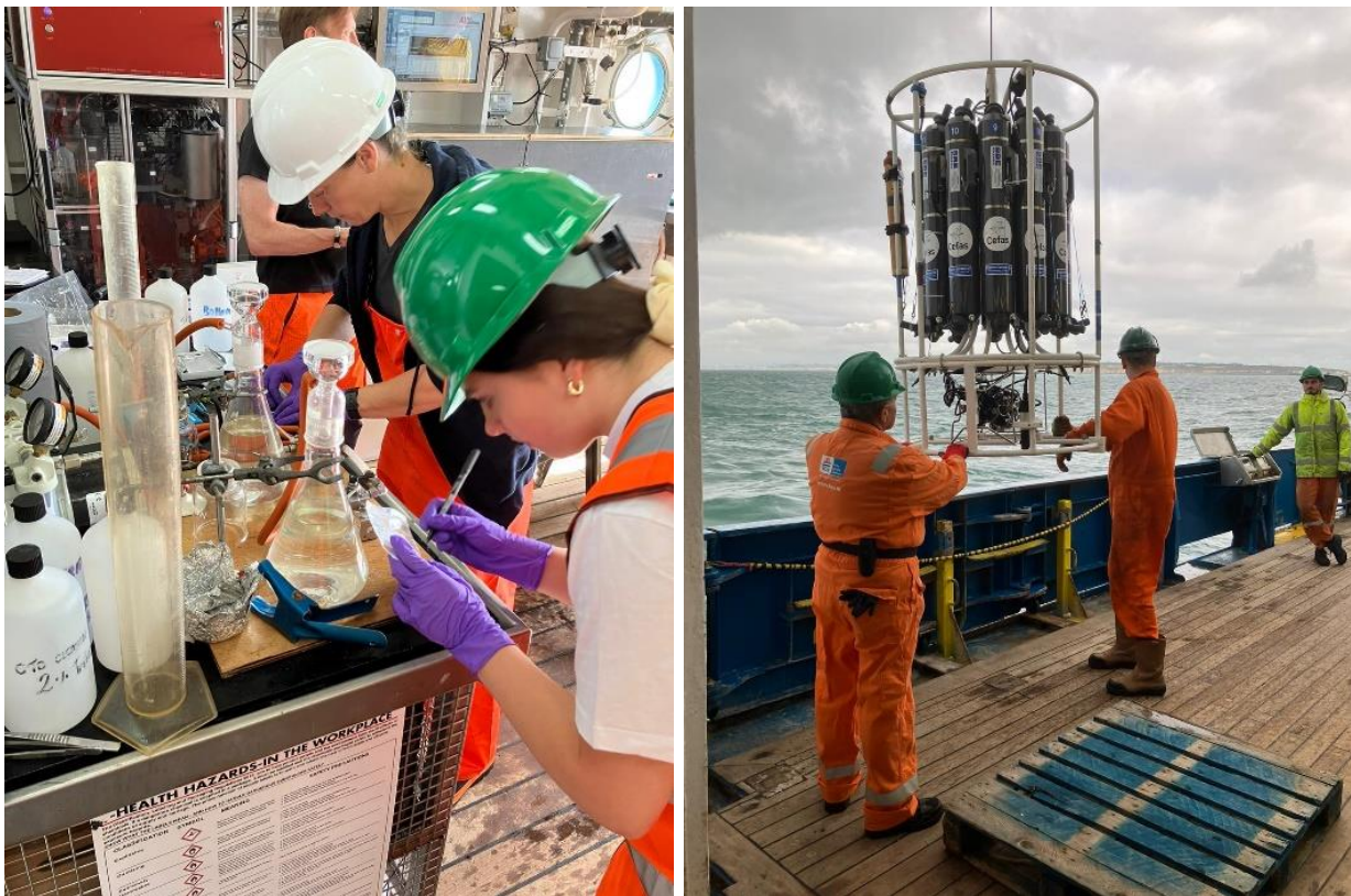
Figure 11: Left - Scientists filtering seawater. Right - Deployment of the CTD Rosette.
