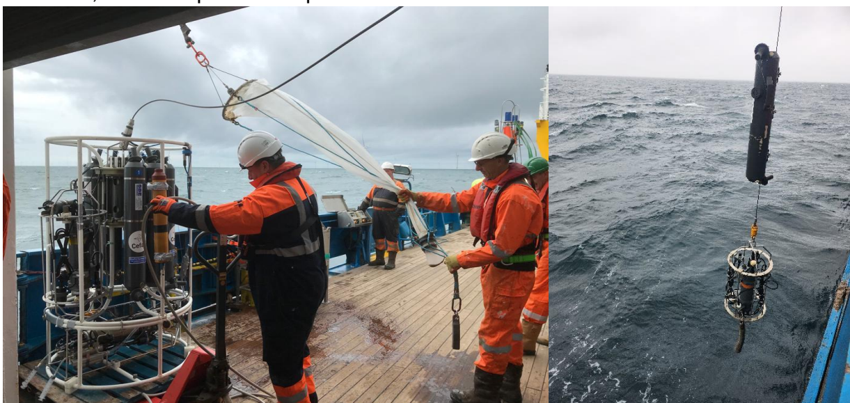
Figure 2. RV Cefas Endeavour deck crew ready to deploy the zooplankton net (left). Also pictured is the CTD Rosette (left) which was not used this survey due to a cabling issue. ESM2 CTD profiler (right) was deployed with a 10 L niskin.
