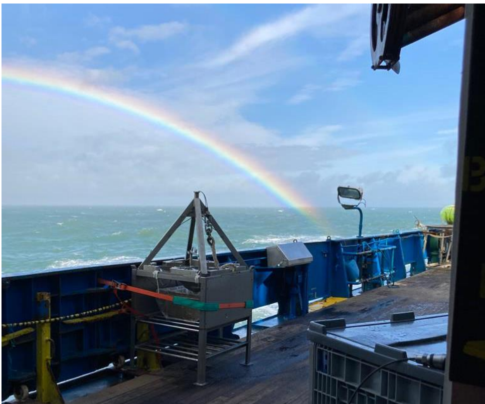
Figure 5. The Day Grab at the side gantry used to collect sediment samples.
