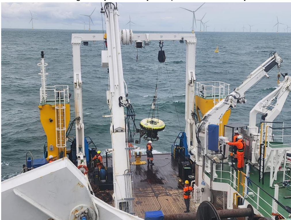
Figure 3. West Gabbard SmartBuoy recovery
