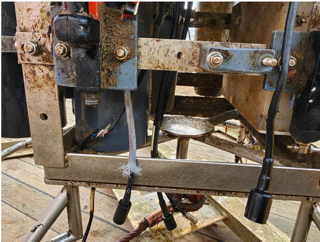
Figure 5. Frayed wires and missing sensors showing damage to West Gabbard Buoy.
