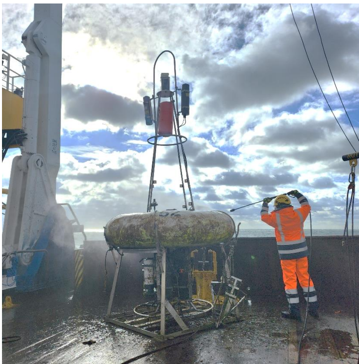
Figure 6. Back deck team jet washing the algal fouling off the SmartBuoy. Note the damage to the licor arm hanging off the right side of the Buoy.
