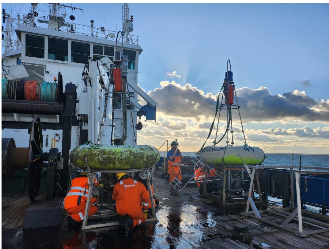
Figure 7. Dismantling of the West Gabbard SmartBuoy by back deck team (Left) and prepping of the Warp SmartBuoy by back deck team (Right). Note the correctly assembled and intact licor arm (Right/Centre).
