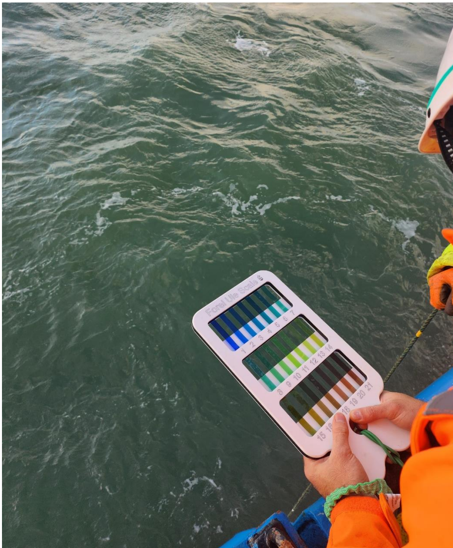
Figure 2. Forel Ule Colour Scale used to observe surface seawater colour for water quality assessments.
