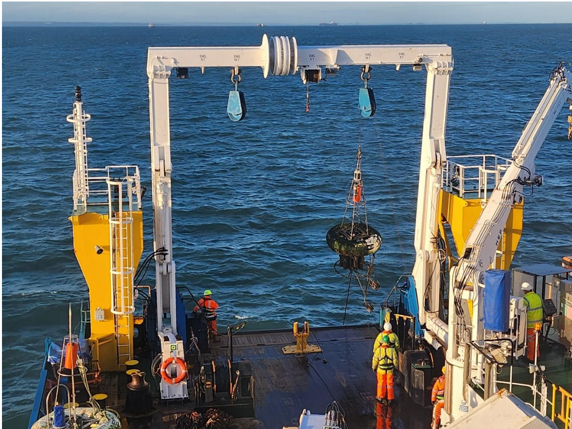
Figure 8. Recovery of the Warp SmartBuoy from the RV Cefas Endeavour.
