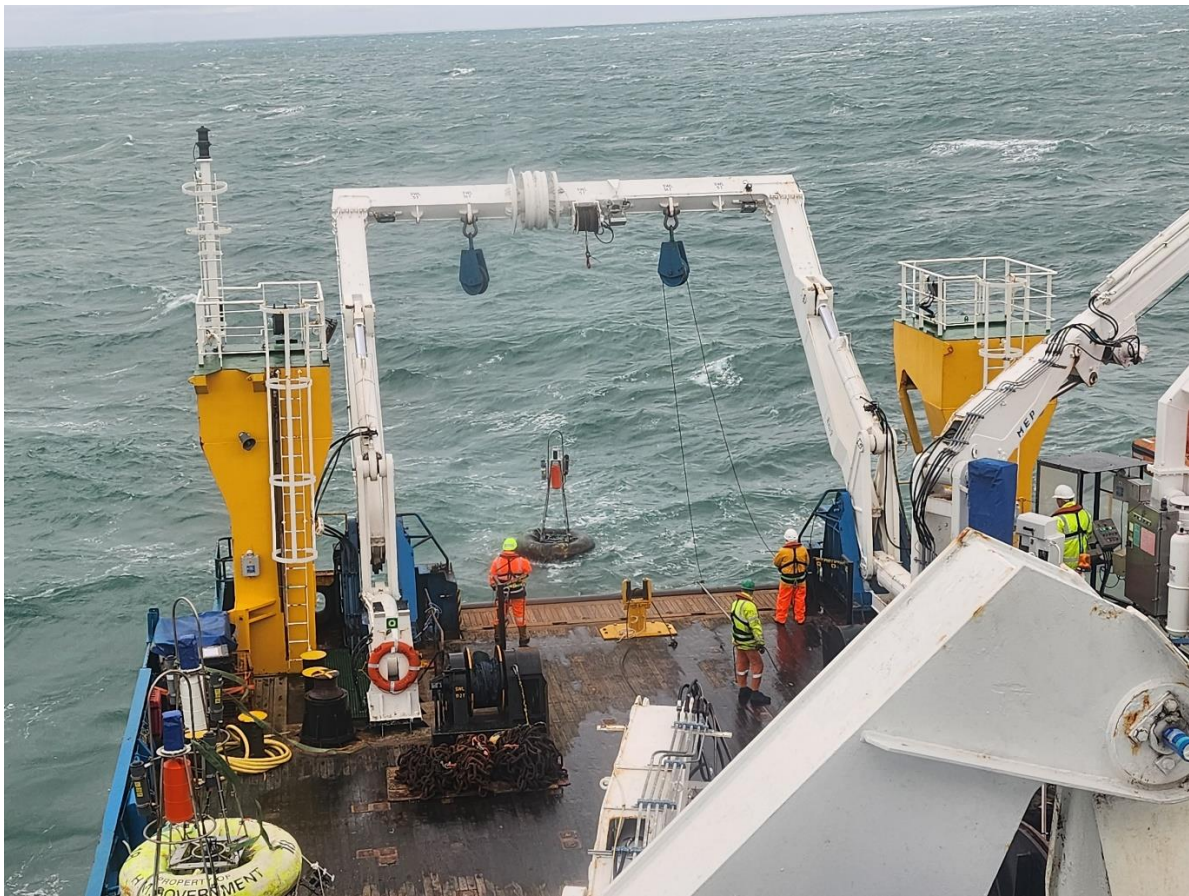
Figure 4. Lowering the A-Frame prior to recovery of the West Gabbard SmartBuoy from the RV Cefas Endeavour.
