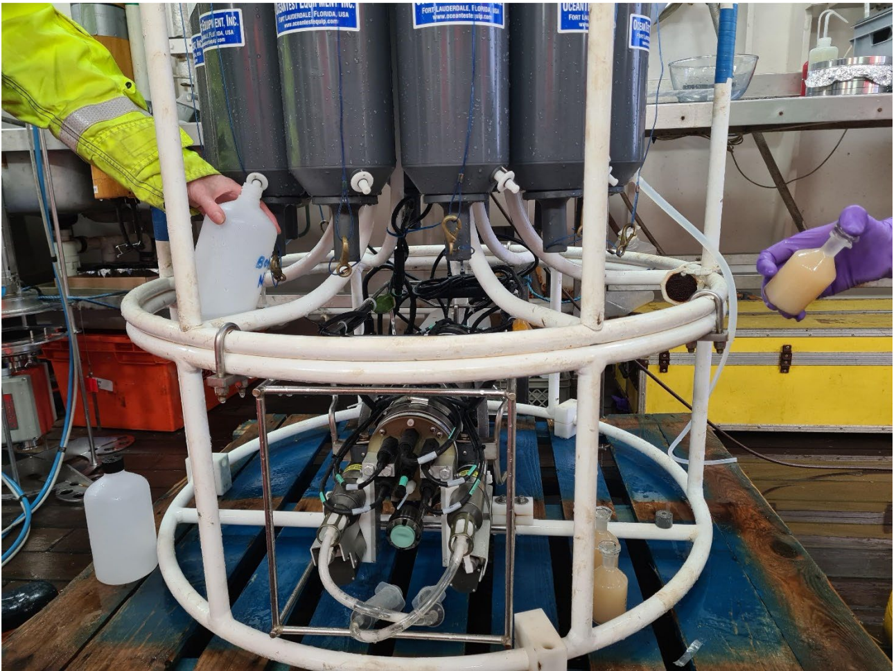
Figure 12: Water samples, including dissolved oxygen samples, being collected from the CTD Rosette from the Smartbuoy site.
