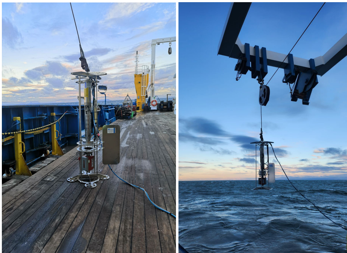
Figure 17: Marine plastics pump left: on deck, right: Being deployed from the side gantry.
