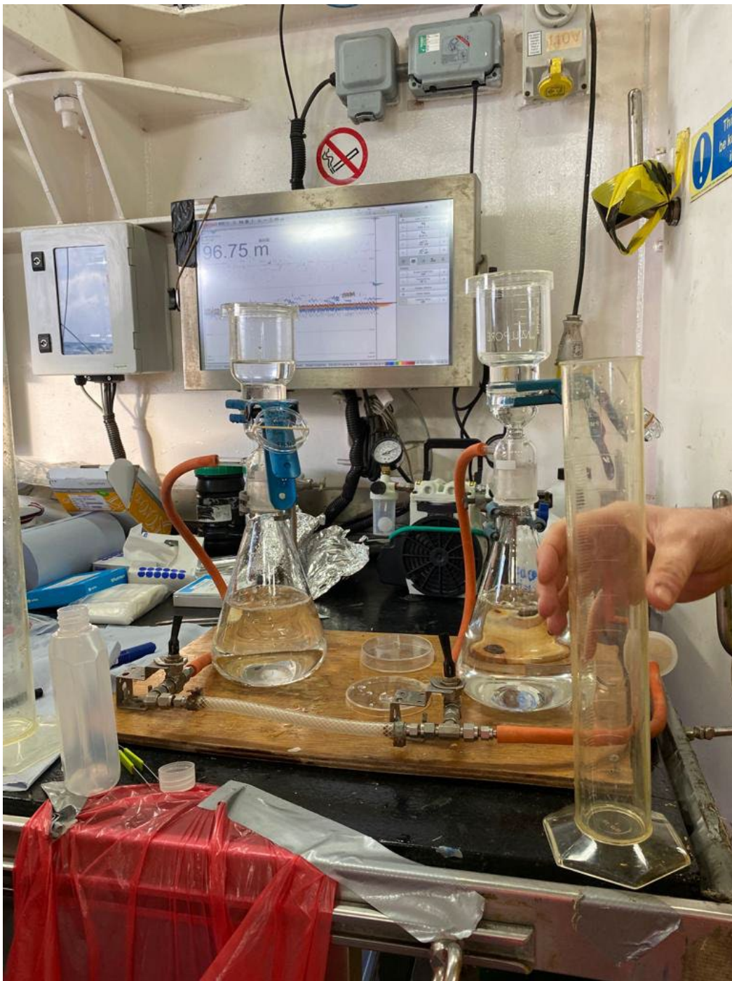
Figure 13: Filtering rig used for filtering out suspended particulate matter and Chlorophyll
