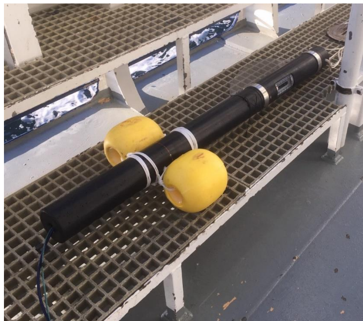
Figure 2: Stereo Catch Monitoring Probe (S-CMP) ready for deployment during the research cruise on M/F Fiskebas. The floatation section and the camera section are connected, with the support line and cable pass through the float so that the depth of the camera relative to the surface can be controlled. This version is fitted with an Ethernet cable, for direct camera feed from the probe, as well as additional weight and floatation to stabilise the camera’s vertical position in the water.
