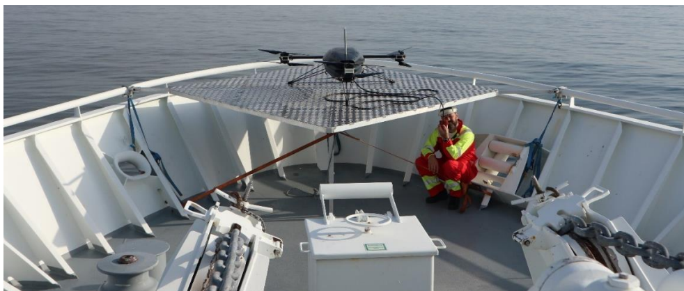
Figure 9: Birdview AS drone with echosounder below is ready for takeoff. The electric winch was not working explaining why Erik Schuster sits under the platform holding the transducer.
