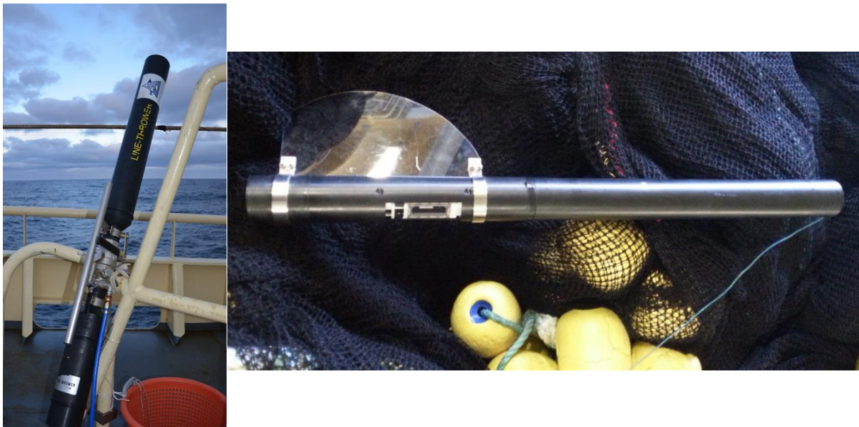
Figure 12: Catch monitoring probe (CMP) in protective housing (right) prepared for deployment from a compressed air canon (left).
