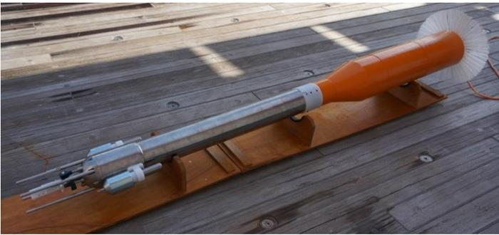
Fig. 7.4.1 Microstructure profiler, TurboMAP-L
