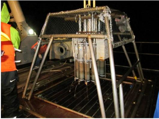
Fig. 1. Photo of the multiple-corer.
