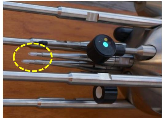
Fig. 7.4.2 Shear probe at the head of TurboMAP
