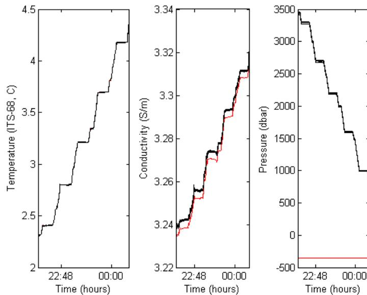
Figure 4: Results from the calibrations dip done between the 24th and 25th September 2011. Each panel includes data from all the microCATs (left: temperature; centre: conductivity; right: pressure). The red curve corresponds to microCAT SBE37-1696, whose pressure sensor was not working and whose conductivity cell gave readings systematically lower than those of the other conductivity sensors.
