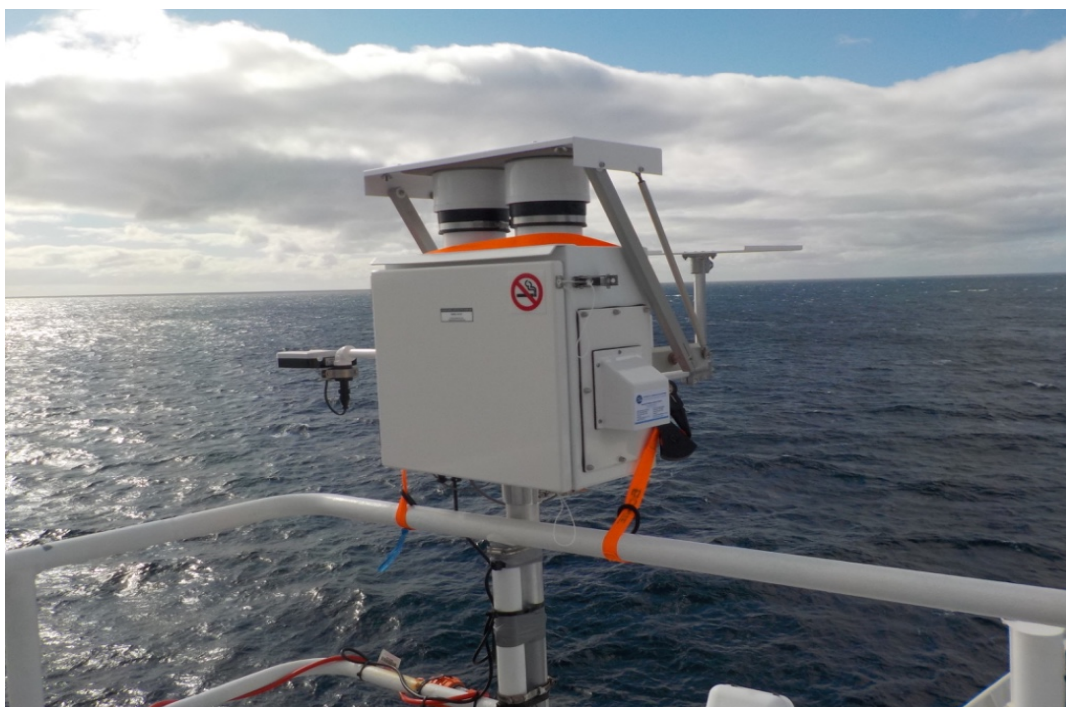
Figure 15. N-CON TM00-127 automatic rain sampler installed on the 5 th deck during INV2016_V04.
