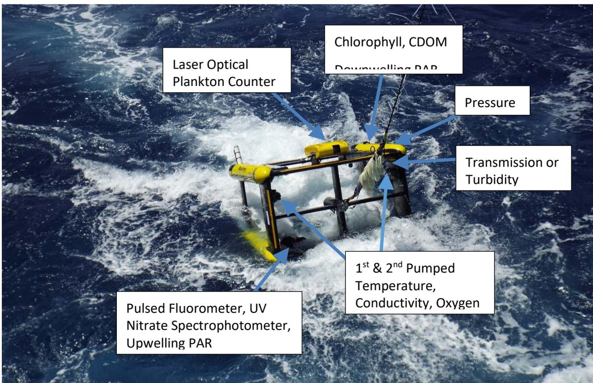
Triaxus undulating towed platform with labelled sensor array.
