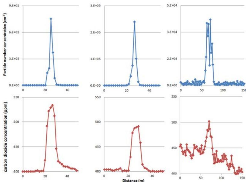
Figure 6 Particle number profiles (top graphs) and CO<sub>2</sub> profiles (bottom graph) collected at 20 m behind the ship and 25 m above the ocean (first 2 columns) and at 100 m behind the ship and 25 m above the ocean (far right graphs).
