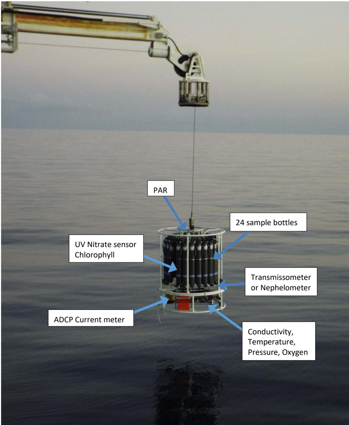
The CTD rosette platform lowers sensors vertically through the water column collecting digital information and, on the up-cast, water samples from selected depths.
