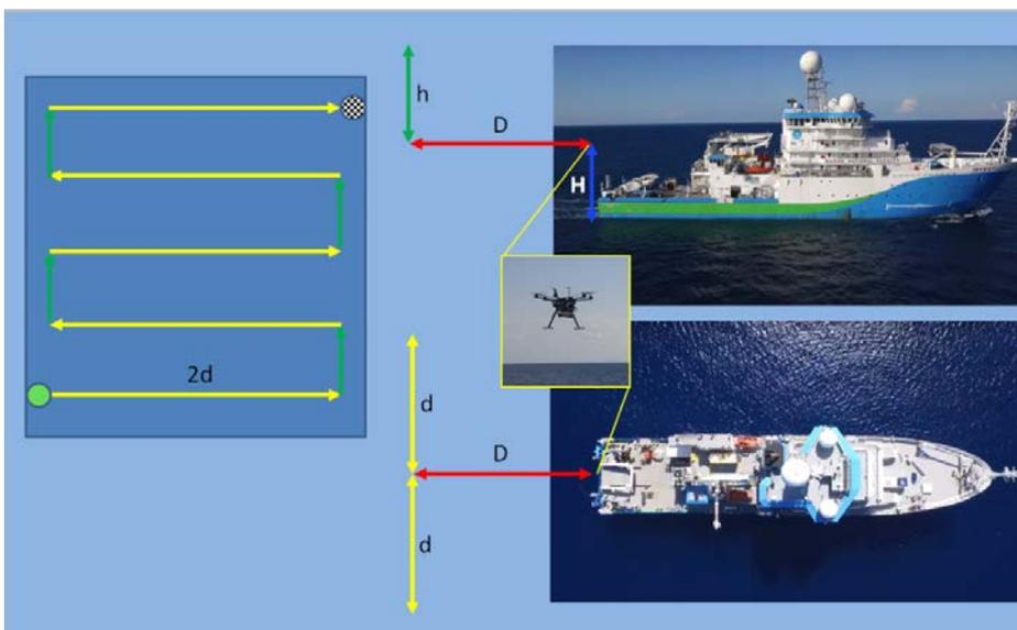
Figure 5 Flight path used to measure the ships diesel engines plume dispersion.
