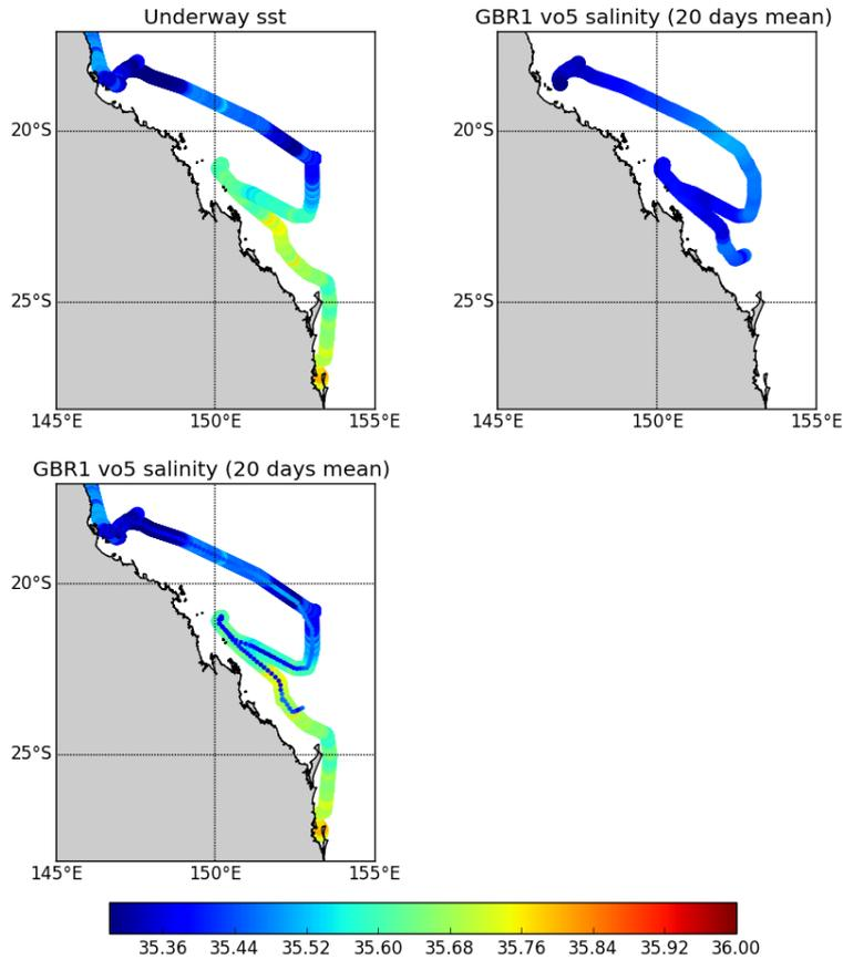
Ship underway salinity (unprocessed, broad line) and simulated surface salinity in the GBR 1km V05 model (using a 20-day average for the model, thin line) generated with script 'ship\_underway\_gbr1Vo5.py'.
