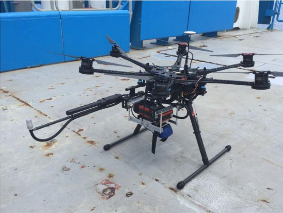
Figure 4 DJI S800 hexacopter with the payload consisting of a Mini Diffusion Size Classifier (DISCmini), to measure the particle concentration, and the Q-trak, to measure the CO<sub>2</sub> concentrations coming from the ship diesel generators.
