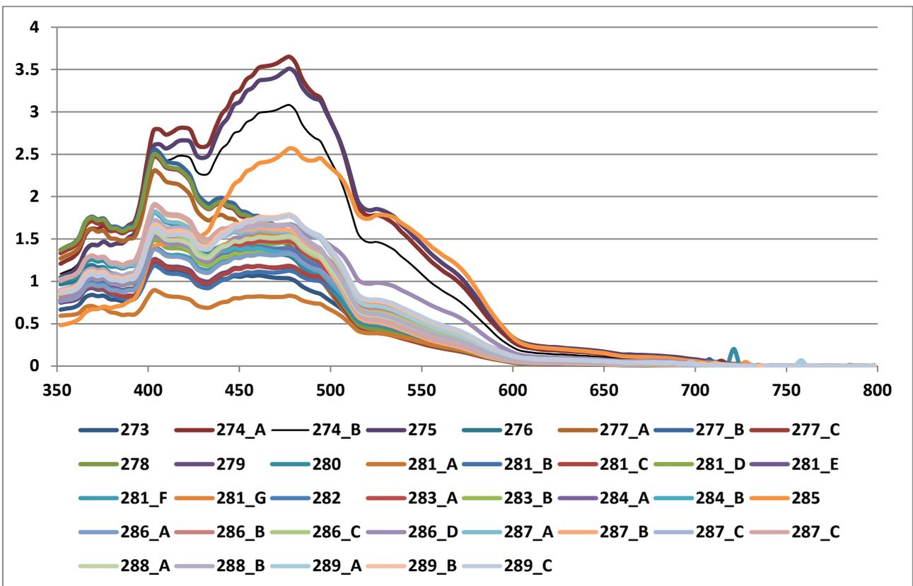
All the spectral water leaving radiance data on the voyage to date. This plot shows the range of water types encountered and cloud conditions at the time of the observation.
