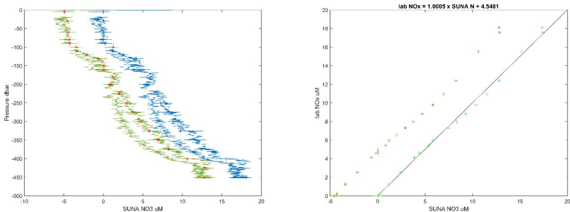
Left figure raw SUNA nitrate (green with red bottle depths on upcast), post processed nitrate (blue with lab nitrate in black). Right figure linear regression (olive green), corrected data (light green) fall on 1:1 line.
