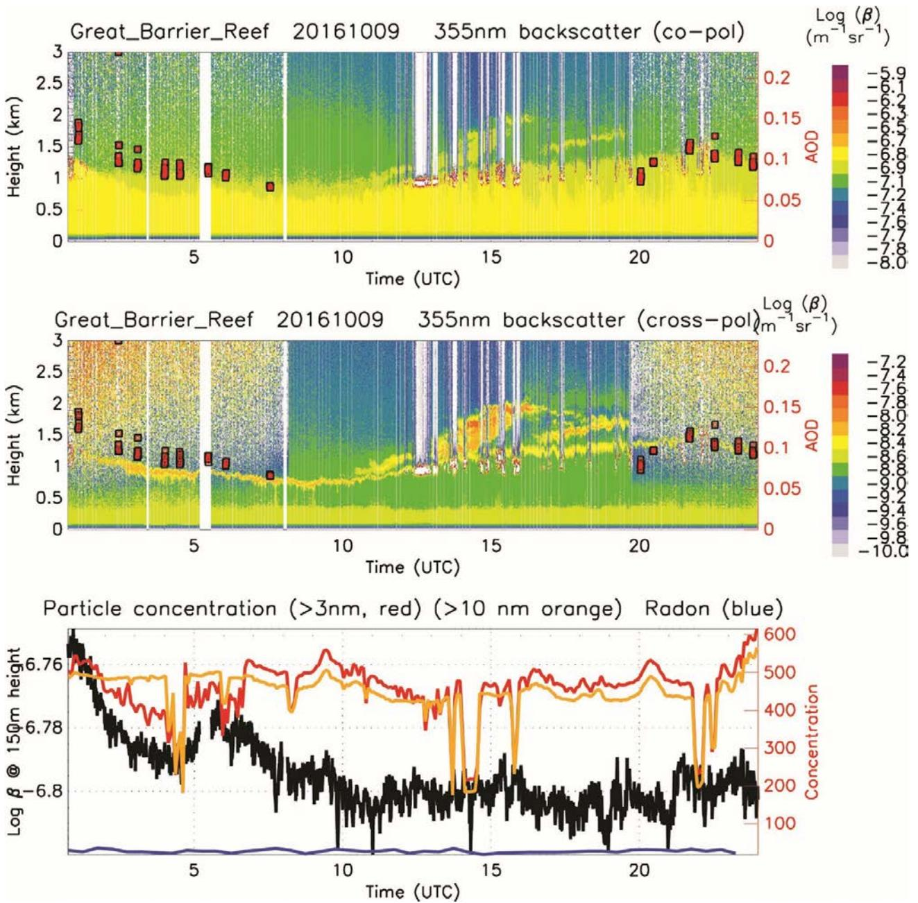
Aerosol optical density as measured with a Microtops hand held sun photometer (red patches) plotted over atmospheric backscatter (from lidar) and particle concentrations as measured on the 9<sup>th</sup> October 2016. Striping denotes strong atmospheric features and contrasting layers of aerosols.
