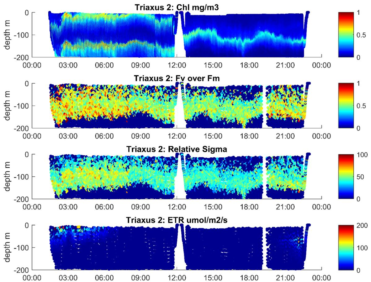
The second Triaxus tow shows the transition from day to night to day. There is a persistent thermocline marking the vertical transition in temperature, salinity, oxygen and nitrate concentration. In the plots of chlorophyll and CDOM the offset between Ecotriplet time/pressure and CTD pressure is clearly shown in the 1<sup>st</sup> segment of the tow. A more realistic subsurface chlorophyll maximum is observed in the 2<sup>nd</sup> segment of the tow.
