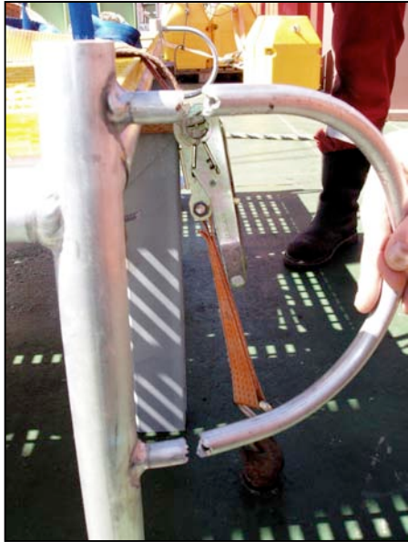
Figure 3 Broken 'grab' on the elevator after impact with the side of the ship.
