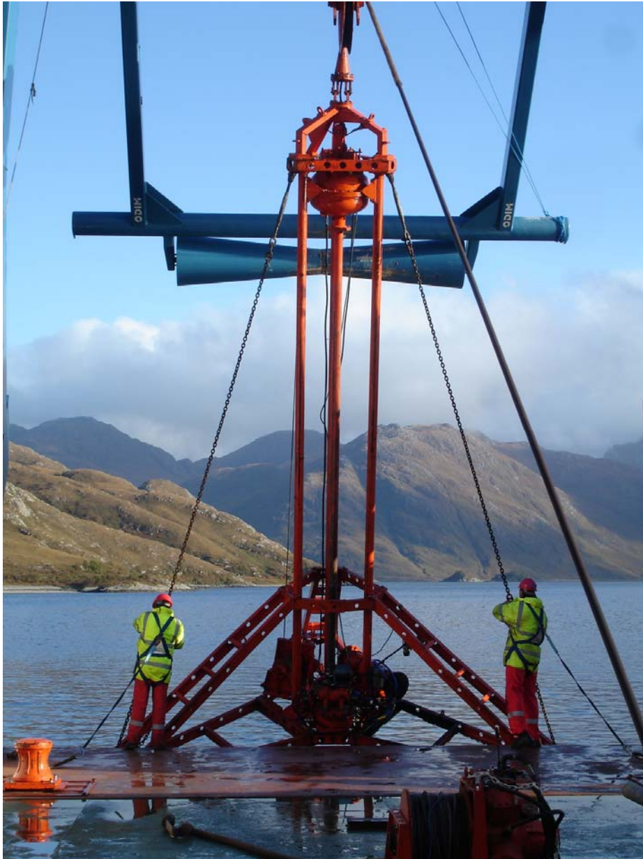
Figure 13 BGS 6m vibrocorer being deployed.
