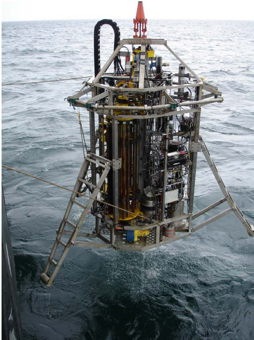
Figure 12 BGS 15m rock-drill being deployed.
